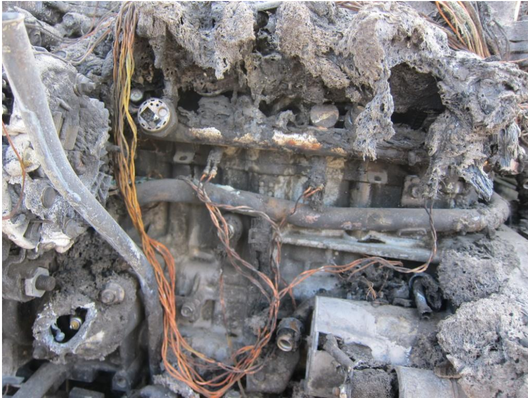
Photograph 11. Flame and heat damage to the front of the engine and fuel injection system.
