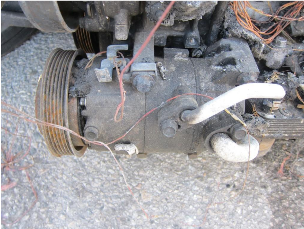
Photograph 13. Air conditioning compressor.
