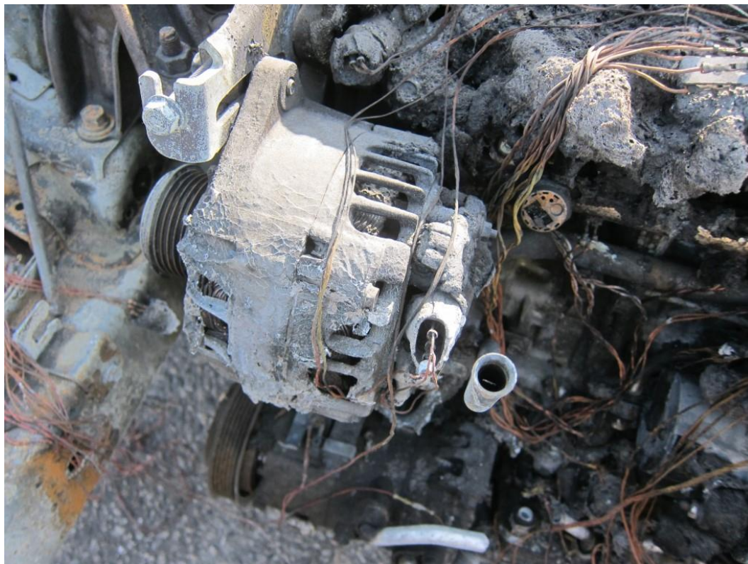
Photograph 25. Close-up of the alternator.
