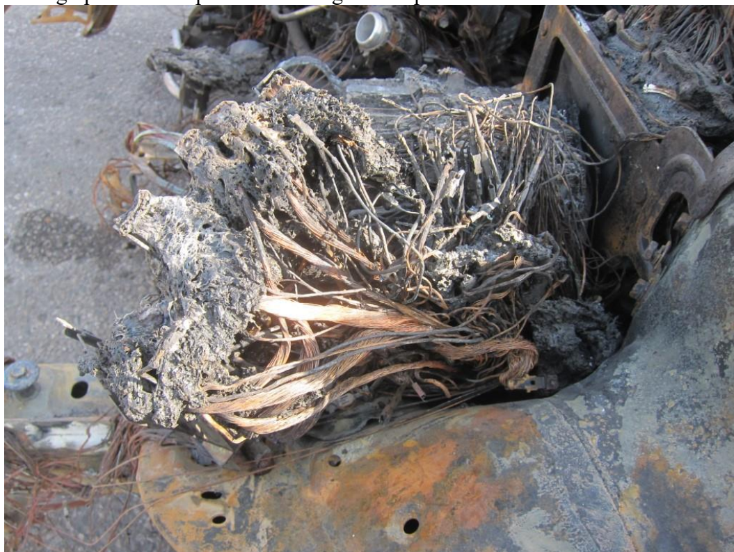
Photograph 22. Underside of the engine compartment fuse box.
