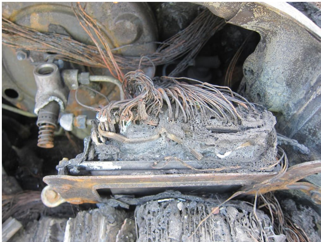
Photograph 29. Close-up of the fire damage to the ECU.
