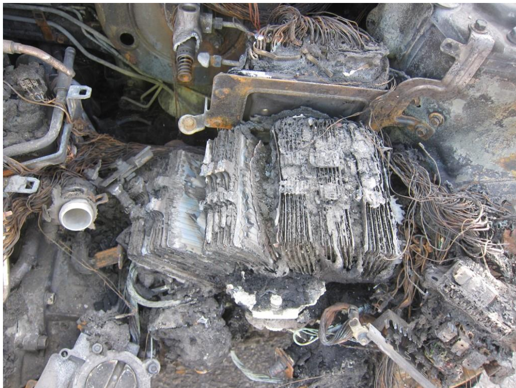
Photograph 19. Condition of the battery as found.
