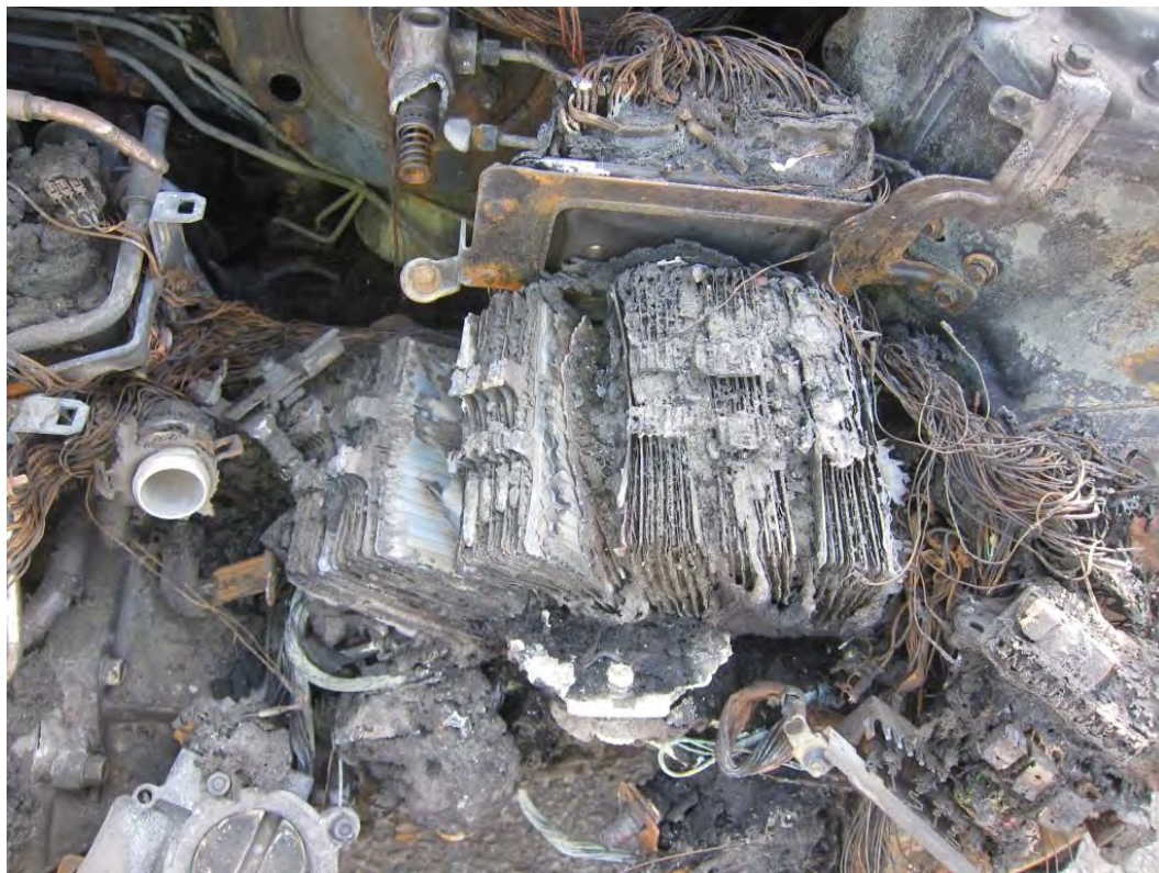
Photograph 19. Condition of the battery as found.
