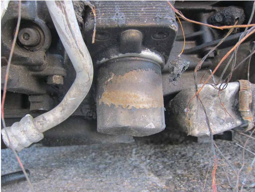
Photograph 17. Condition of the engine oil cooler and oil filter.
