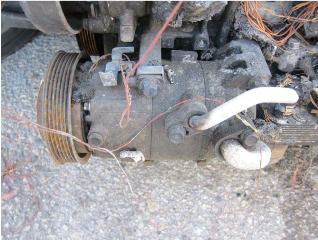
Photograph 13. Air conditioning compressor.
