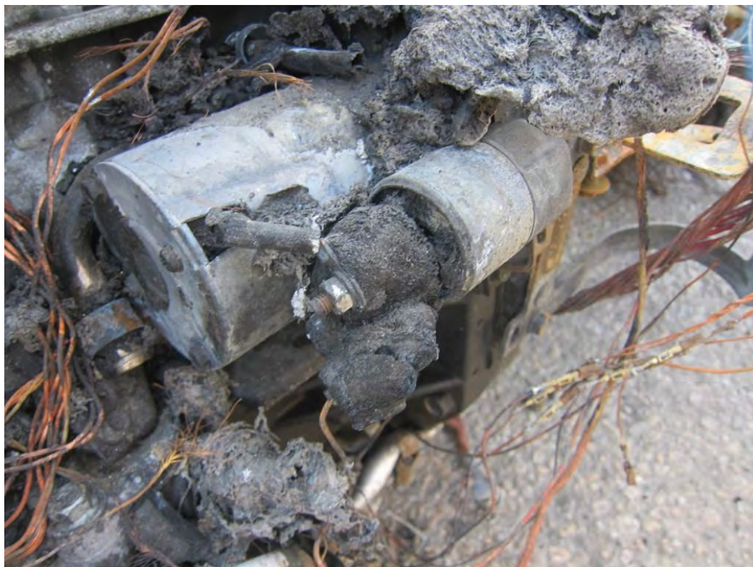
Photograph 24. Close-up of the starter.
