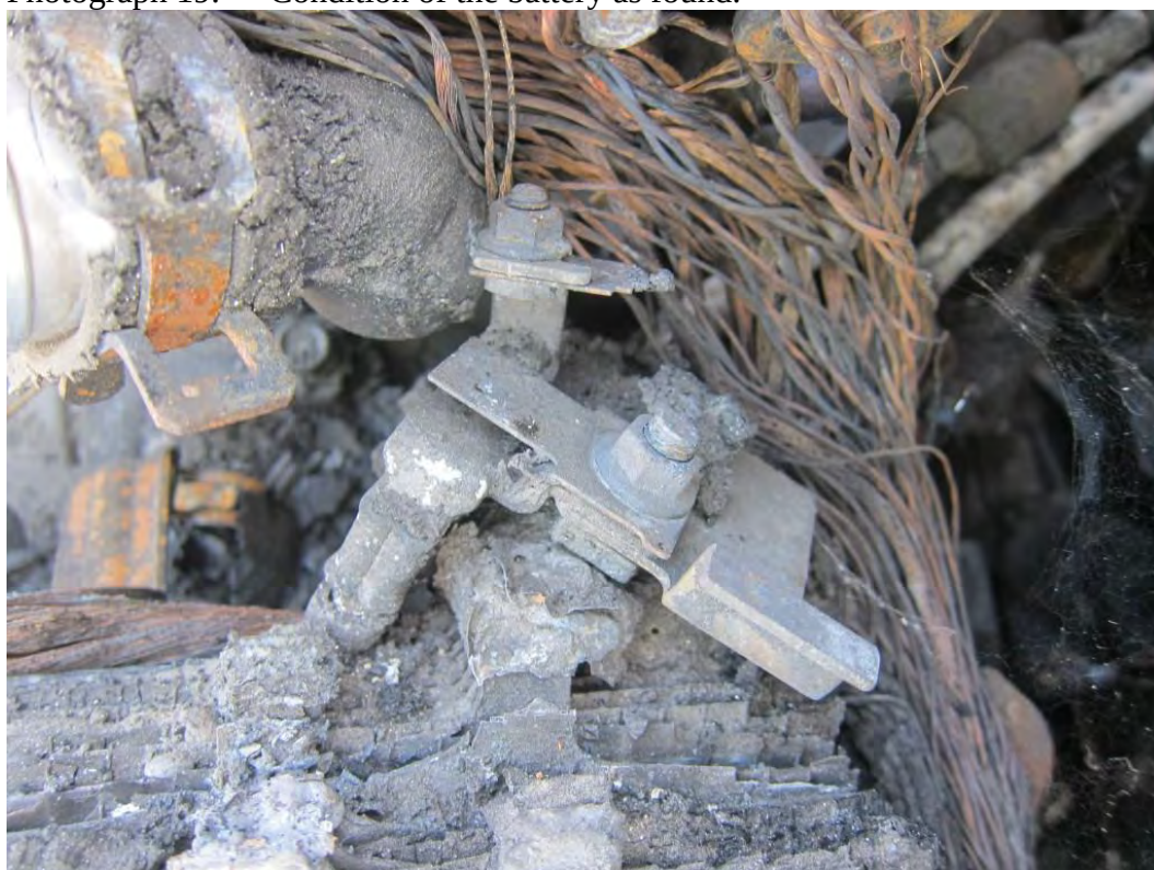
Photograph 20. Close-up of positive battery cable terminal.
