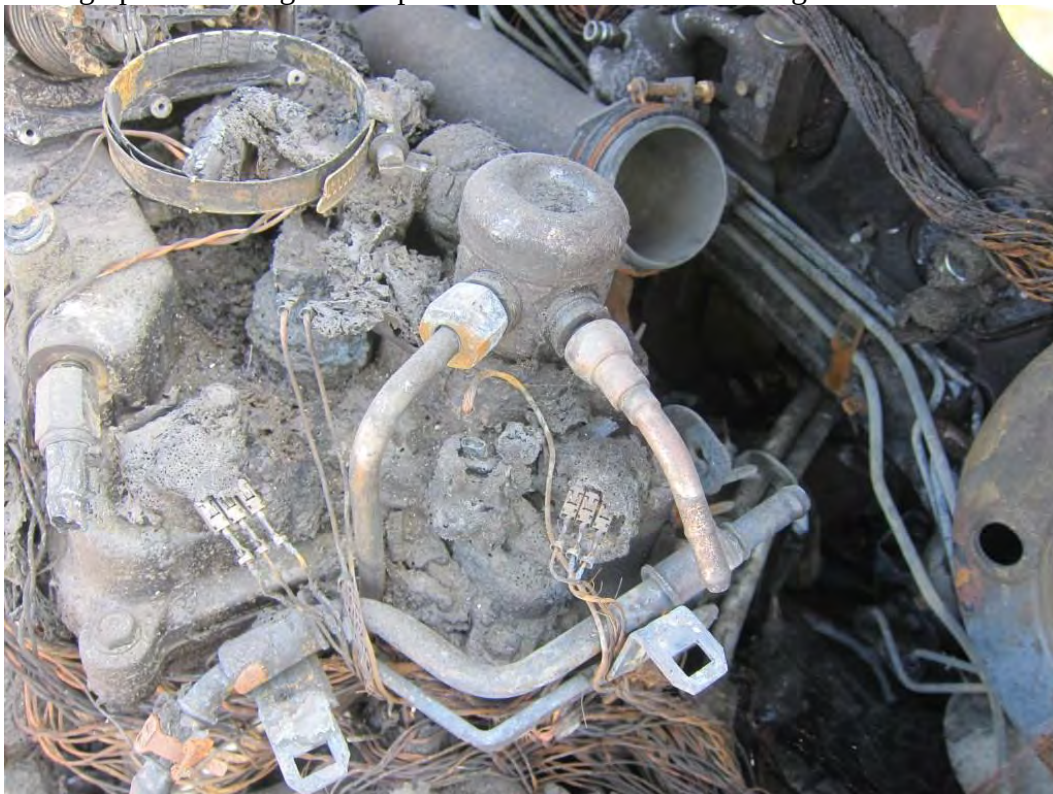
Photograph 10. High-pressure fuel pump.
