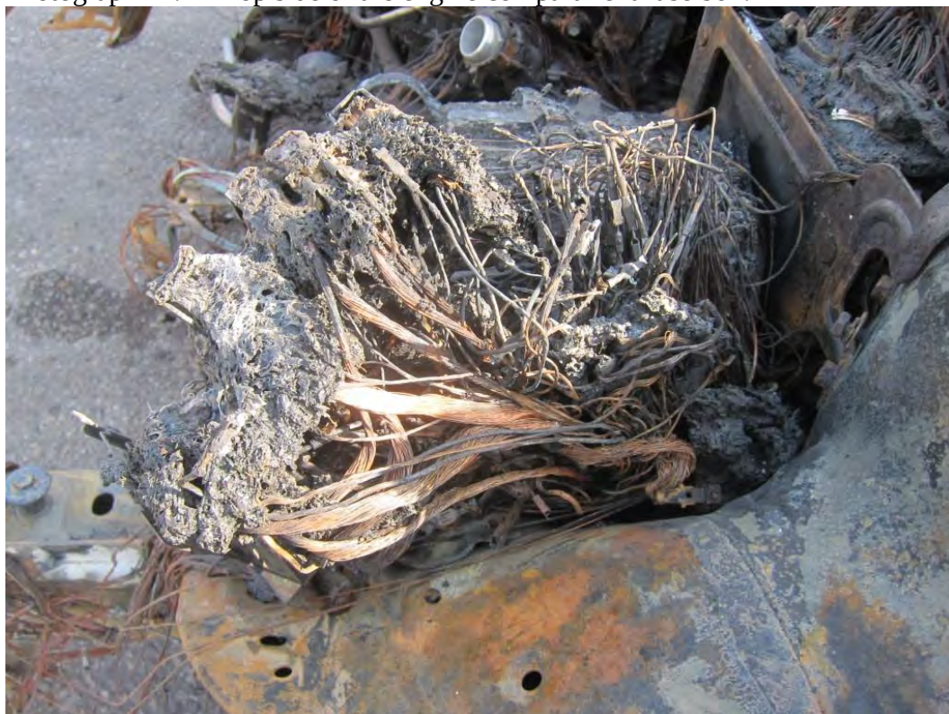
Photograph 22. Underside of the engine compartment fuse box.
