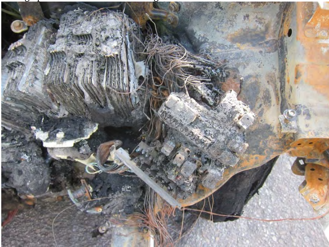
Photograph 18. Area of origin of the fire at the left front of the engine compartment.
