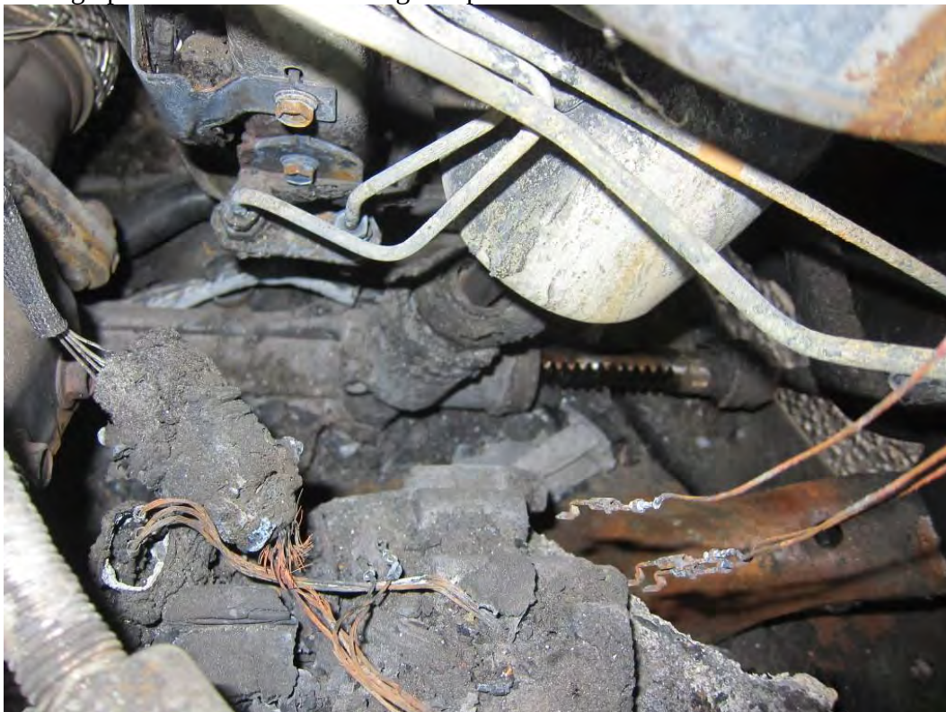
Photograph 14. Left side of the steering rack and the lower end of the steering column.
