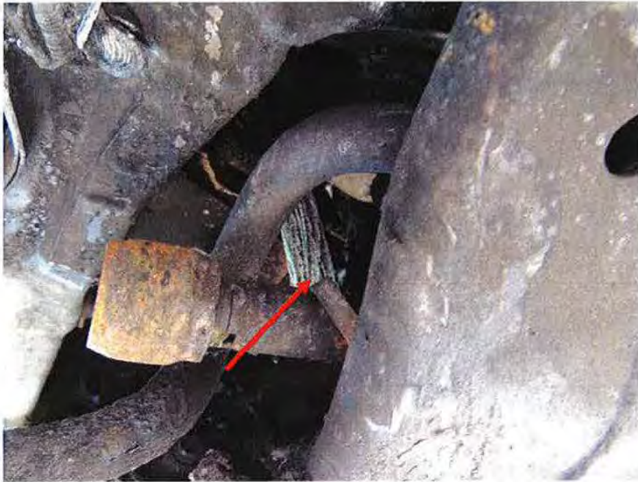
11 Undercarriage of the engine the red arrow depict the corrosion on a wiring harness
