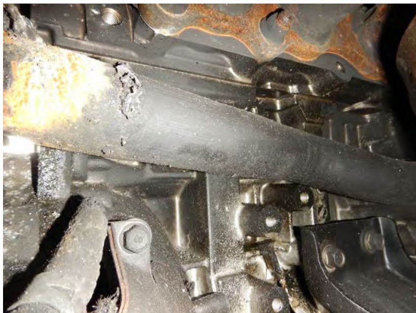
Photo No. 32: Rear exhaust system and oil residue from rear engine block rupture
