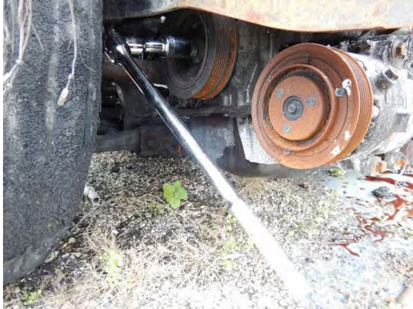
Photo No. 31: Crankshaft would not rotate
