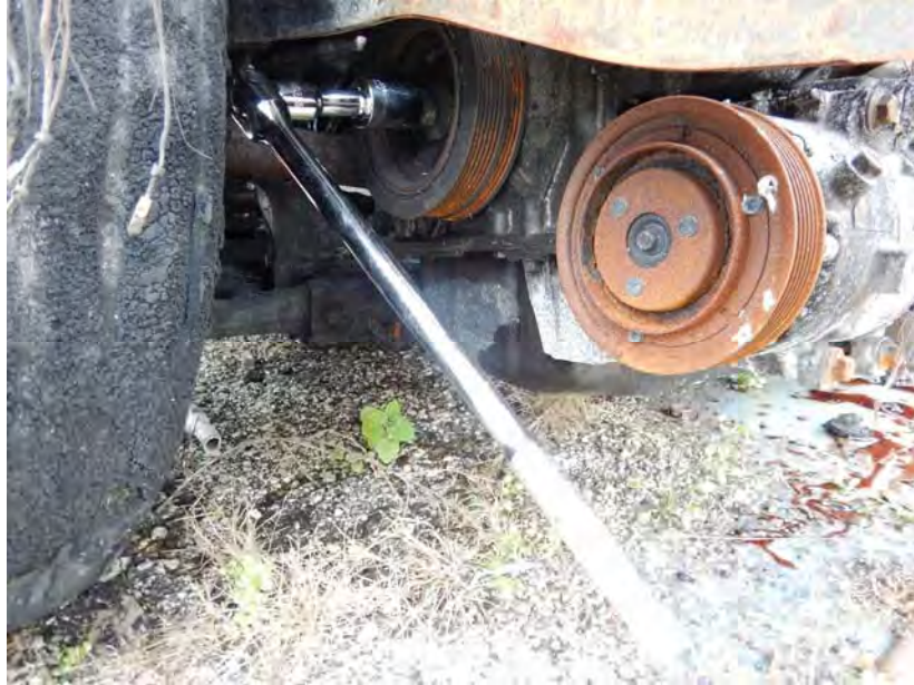
Photo No. 31: Crankshaft would not rotate
