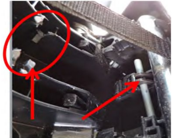
Figure 5 Housing Fractured and Pin in Latch
