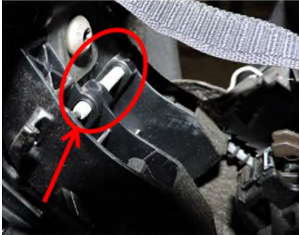
Figure 4 Housing Intact and Latch Pin in Housing
