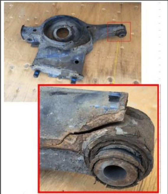
Figure 8. Sample Part with Corrosion at Bushing and Bead Weld
