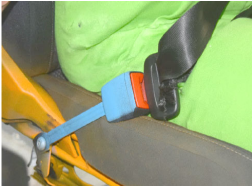
Figure 06: Strap position driver side, light bunching, Damage to the belt strap in the front area
