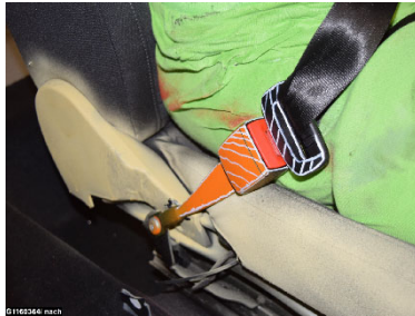
Figure 03: Belt position driver's side, minor bunching
