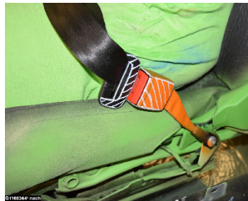
Figure 04: Seat belt position passenger side, minor bunching
