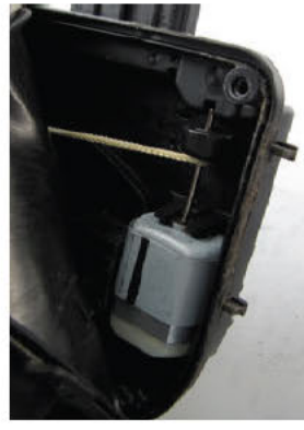
Latch received with 1 winding left on the motorshaft
