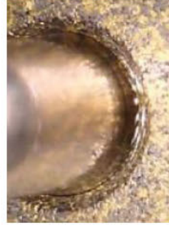
Play between shaft and bearing
