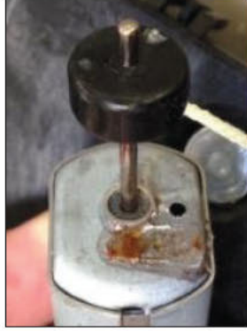
Corrosion visible at motor housing, sinter bearing grey
