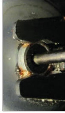
Sinter bearing grey, corrosion on motor housing visible
