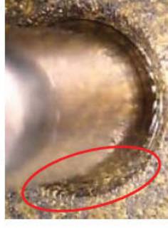
Forced contact shaft is pulled against bearing
