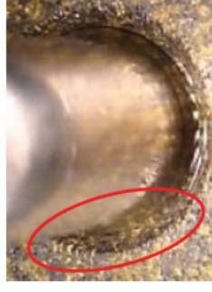
Forced contact shaft is pulled against bearing
