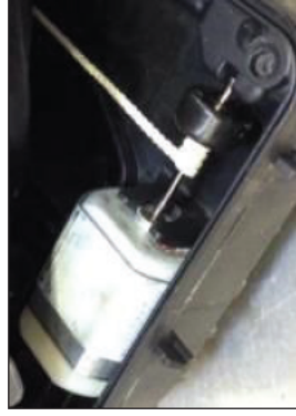
Latch received with 3 windings left on motor shaft
