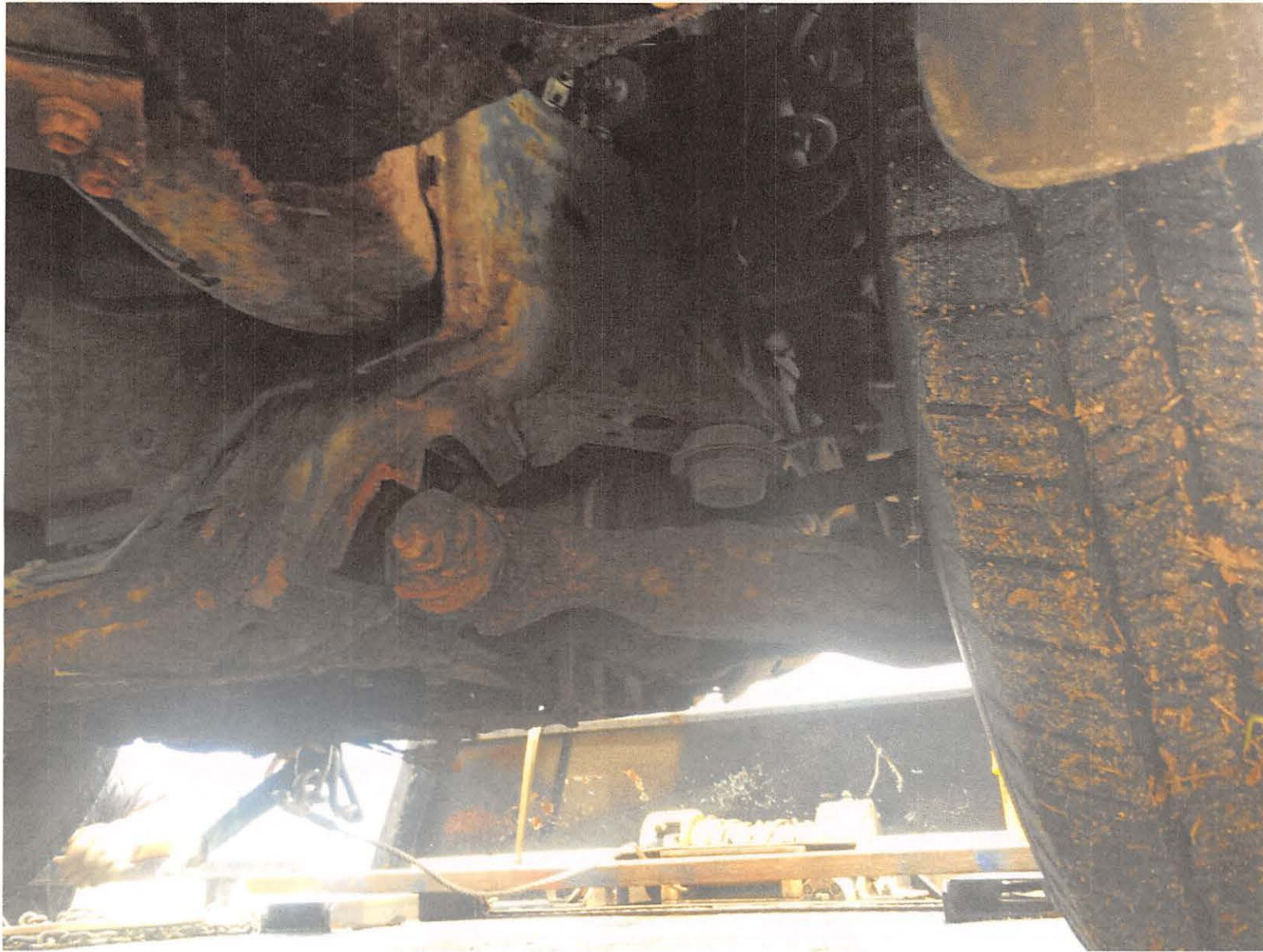
Figure 2 - This photo shows where the steering/suspension system separated from the frame while driving at highway speed.
