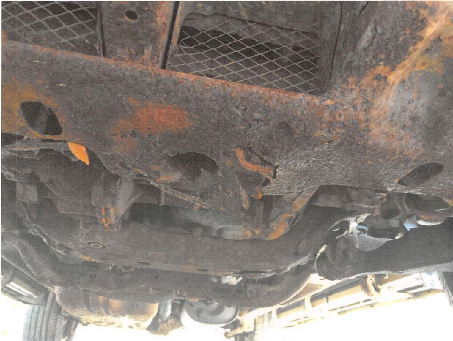
Figure 3 - The steel in the frame could have been properly protected by Toyota. Notice the condition of the original muffler. Absent effective corrosion protection, the frame is clearly not roadworthy.
