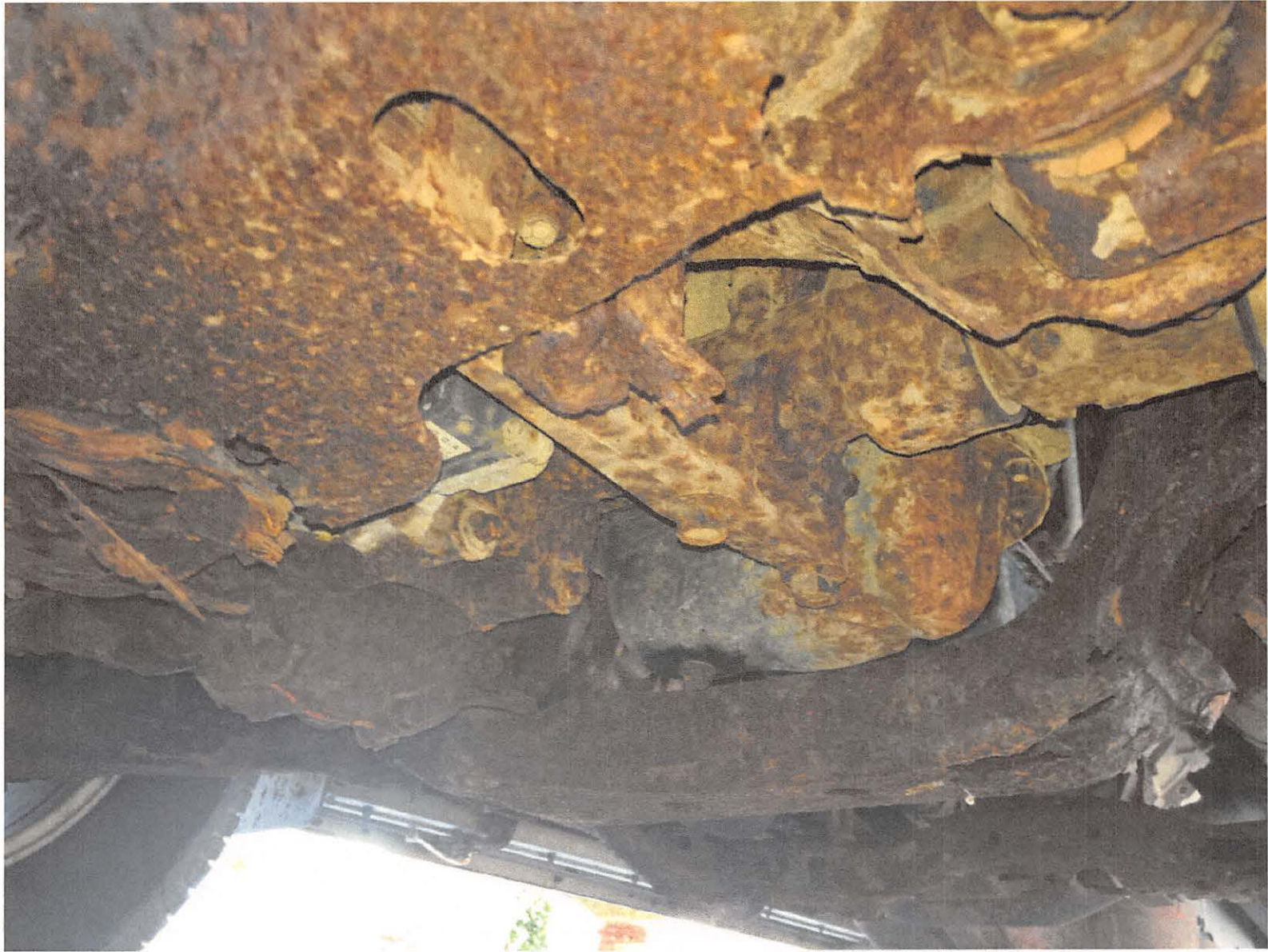
Figure 4 - This vehicle has never been operated in northern states where road salt is applied.
