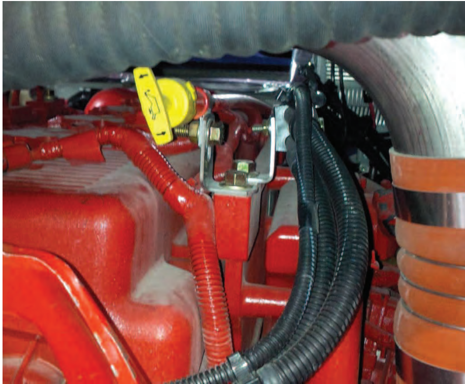
Figure 1: Typical brackets to be tested with the Impact Hammer
