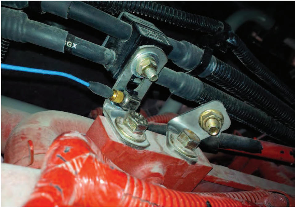
Figure 3: Brackets #4 ("twisted") & #5 (with accelerometer installed)
