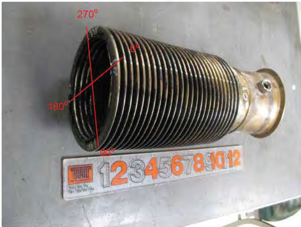
Figure 2 Close up view showing the primary fracture surface with orientations that shows all cracking was concentrated in the 270° quadrant.
