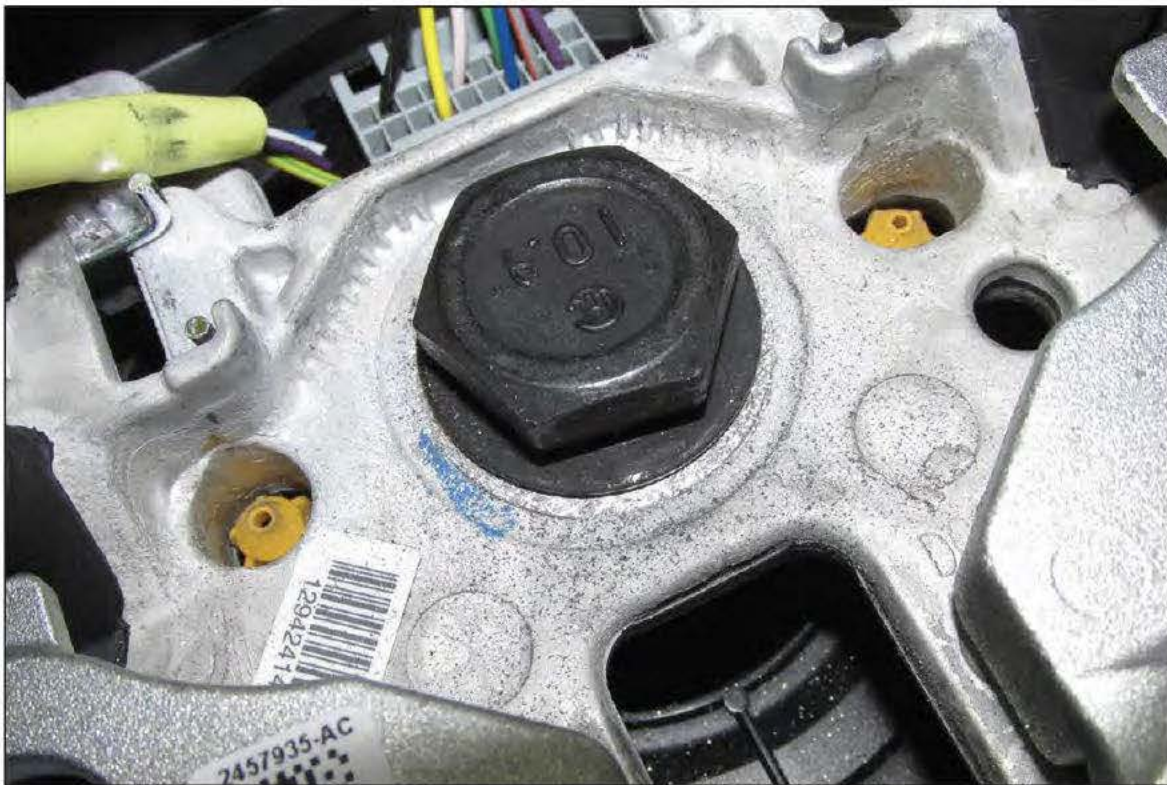
Retaining bolt as found, and shadow illustrating amount bolt was loose.
