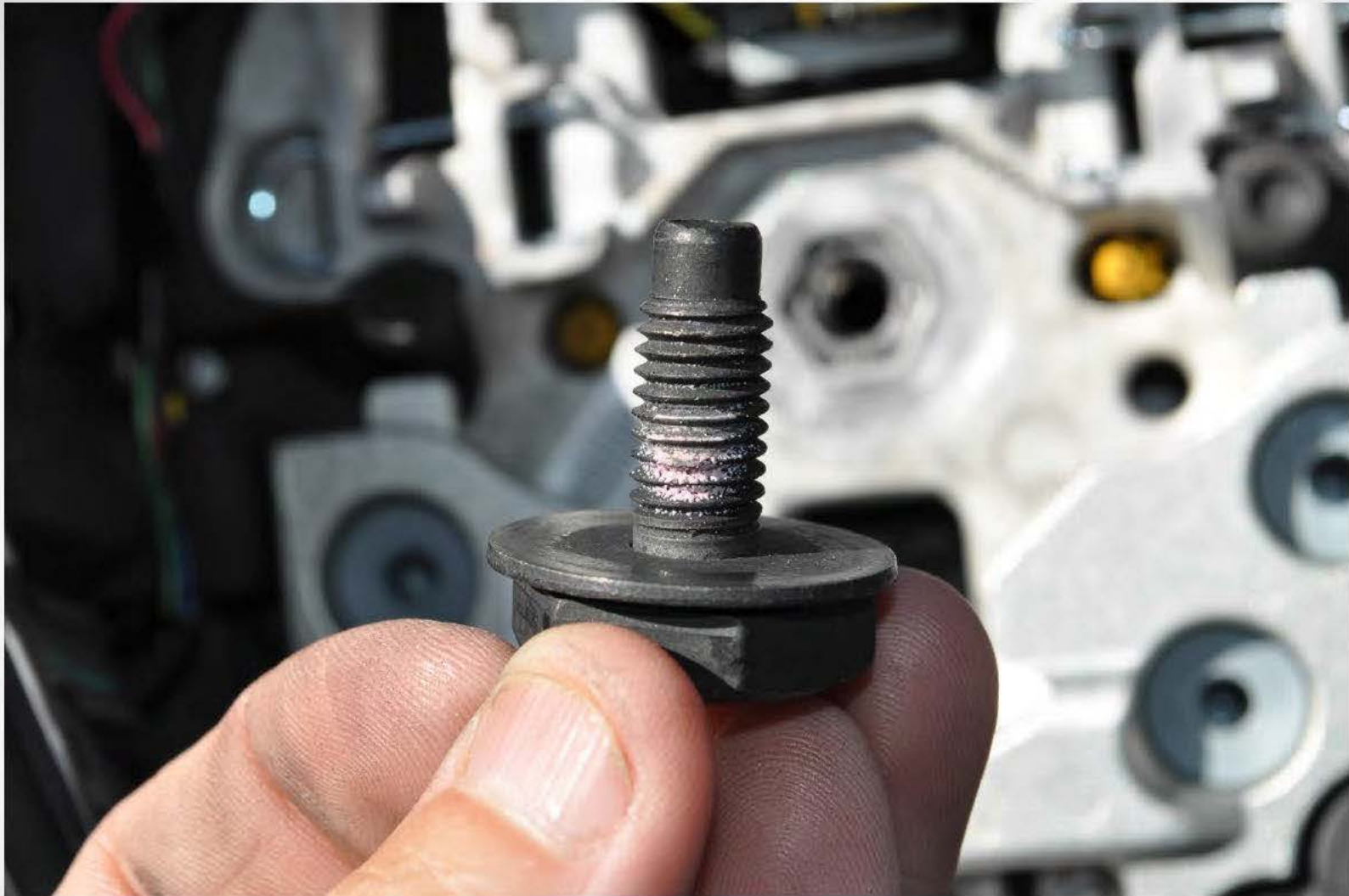
Subject vehicle bolt showing “locking” patch
