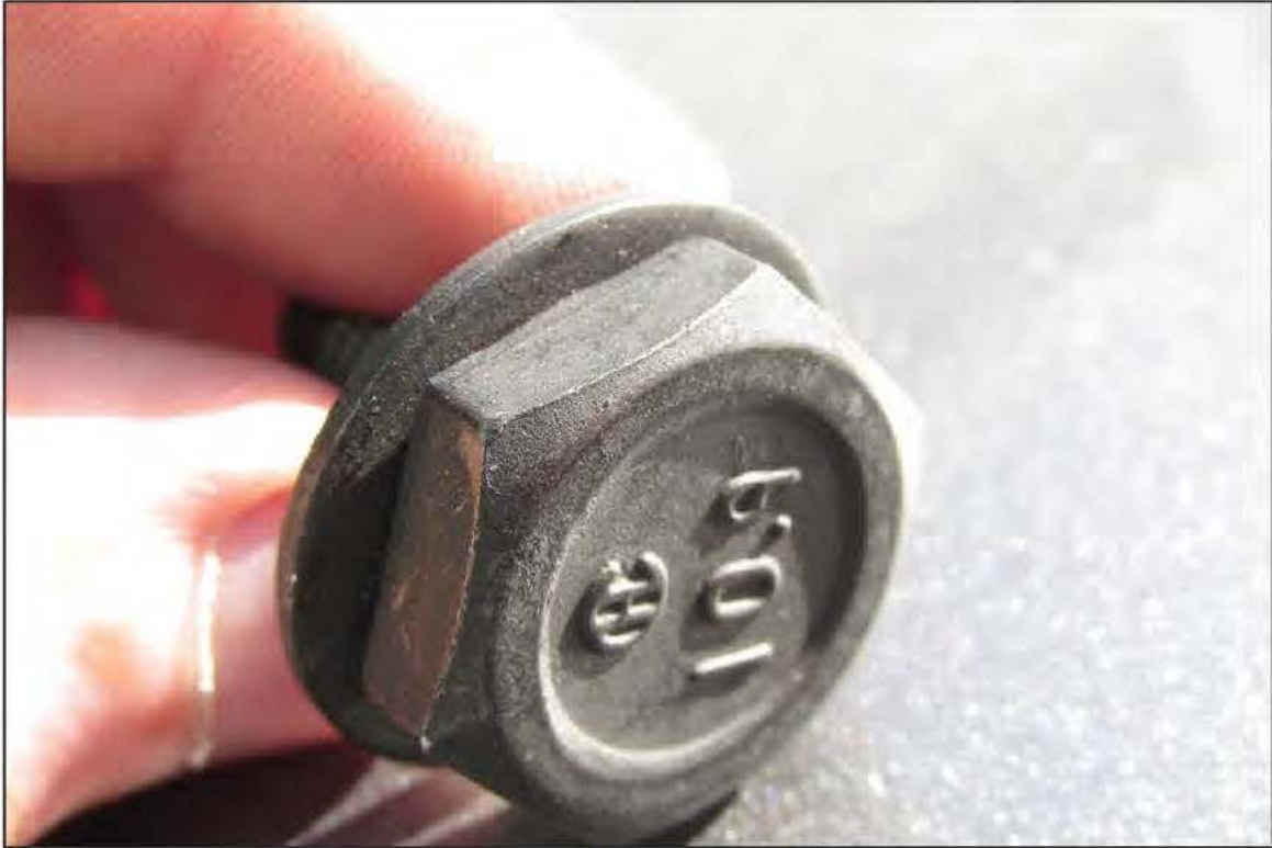
Close-up of the retaining bolt.
