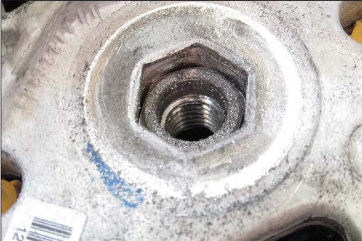
Steering wheel base, with uneven wearing around washer area of the bolt.
