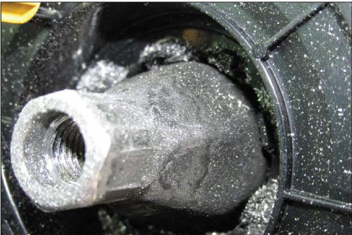
Steering column wear and aluminum particles.
