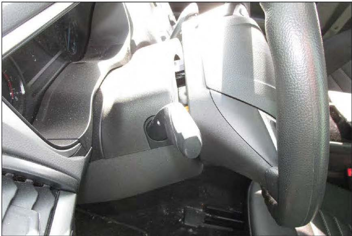
View showing large gap between wheel and column.
