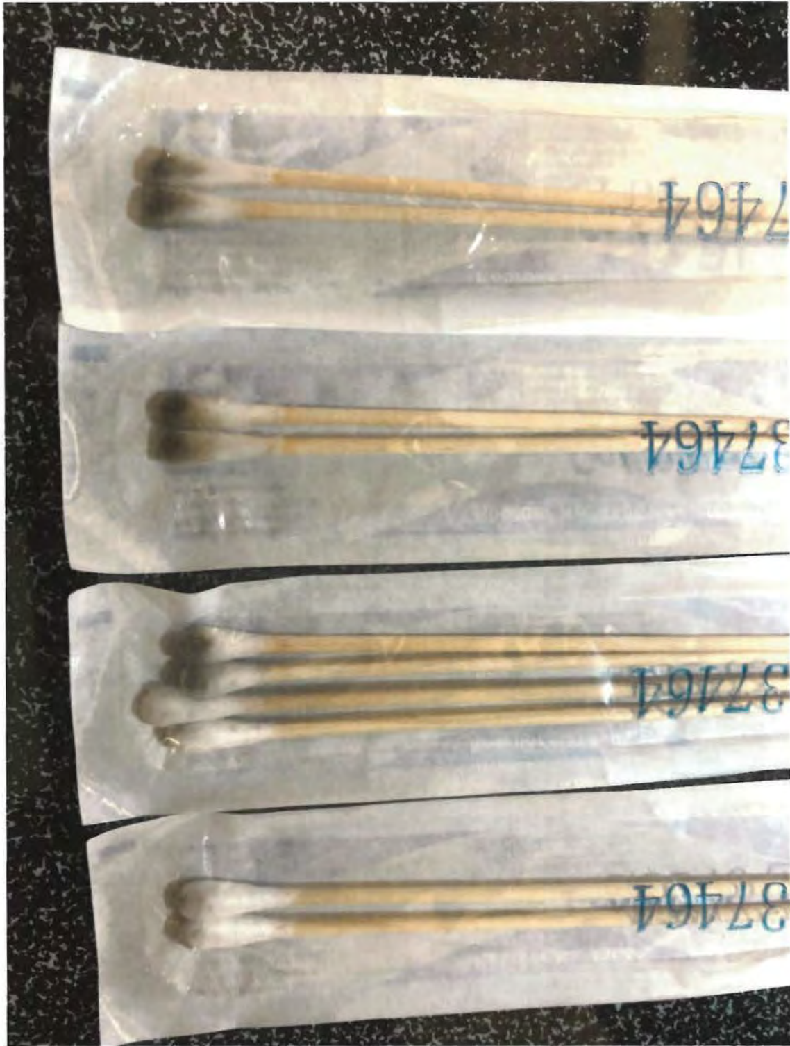
Fig#7: Black residue from the interior AC vents.
