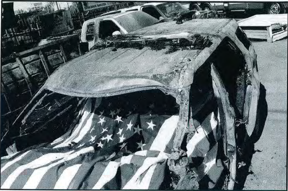
The damage to the roof of Vehicle 1 (Ford) at the scene. CL-012-17 05-13-17 RS-A (285) cropped
