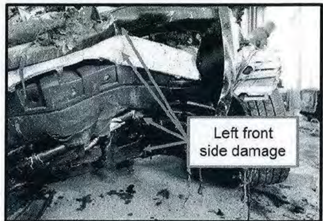
The damage to the left front side of Vehicle 1 (Ford). CL-012-17 05-13-17 RS-B (49)
