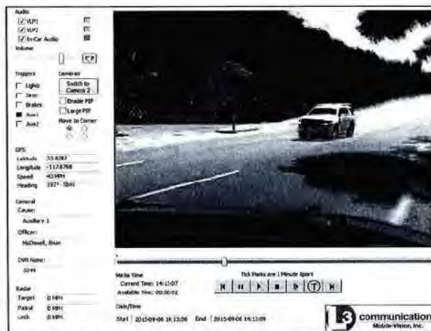
Figure 32. At time 1413:07 hours, the left-front tire of the Ford had dismounted the east curb of the median
