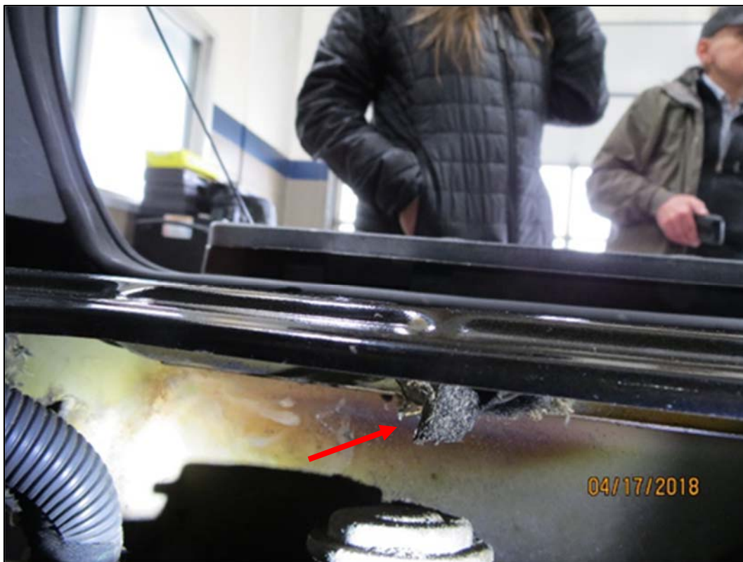
Figure 6. Burned insulation in 2008 Smart Fortwo involved in non-crash engine compartment fire.
