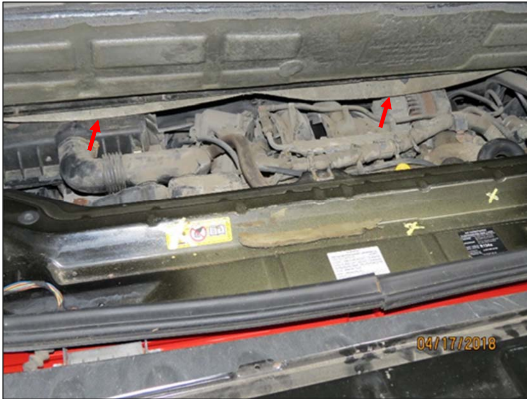
Figure 5. Insulation sagging in 2008 Smart Fortwo involved in non-crash engine compartment fire.
