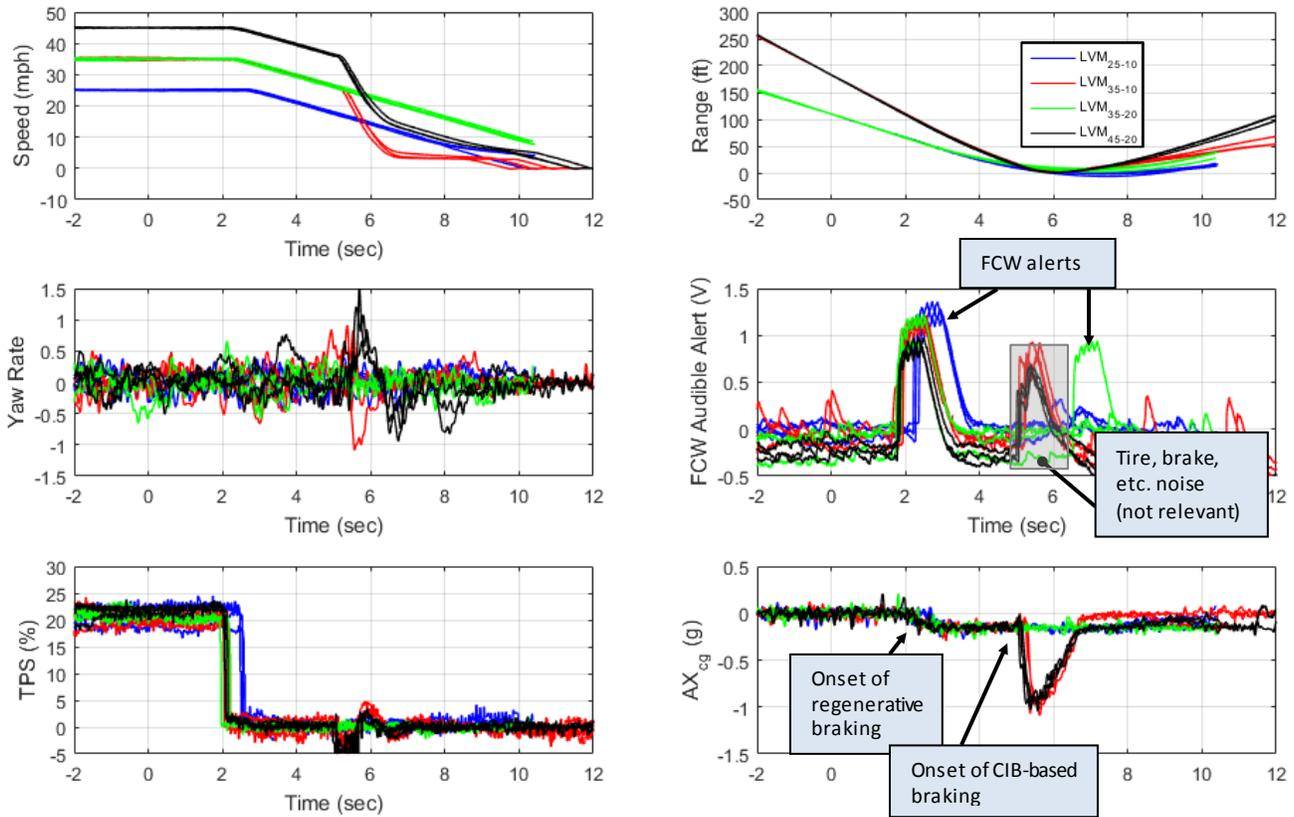
Figure 19. LVM tests performed with the Tesla Model S. Multiple FCW alerts occurred during one of the LVM\_35\_20 trials.
