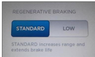
Figure 6. Tesla Model S regenerative brake settings. Selection is available from a menu on the center display touchscreen.
