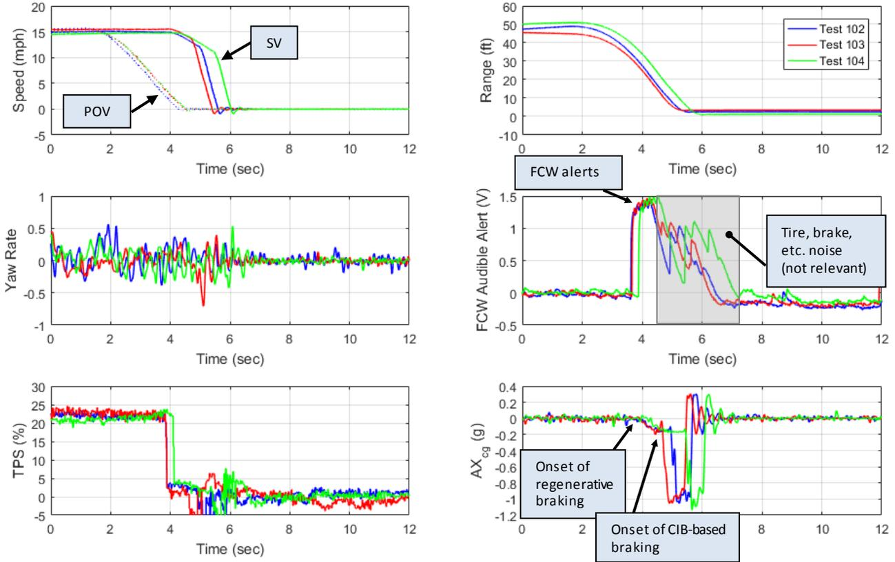
Figure 22. LVD\_15\_15 tests performed with the Tesla Model S.
