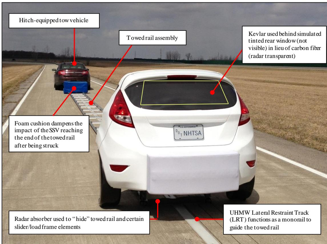
Figure 8. Important design elements of NHTSA's SSV
