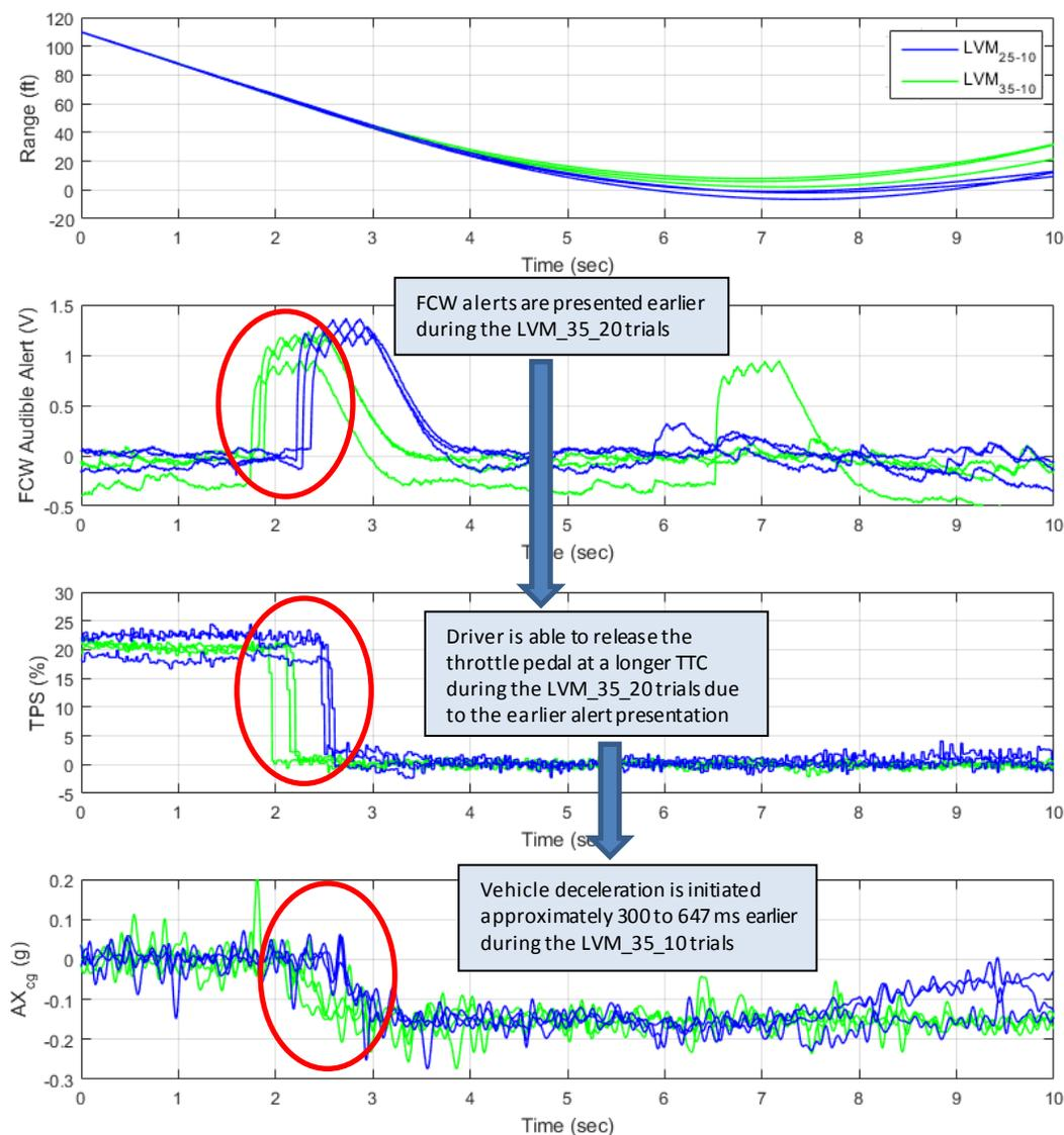
Figure 20. LVM tests performed with the Tesla Model S and a 15 mph relative SV-to-POV speed.
