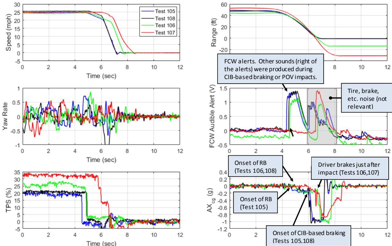
Figure 34. LVD\_25\_25 tests performed with the Tesla Model S (no ACC or LCC). Note: “RB” = regenerative braking.
