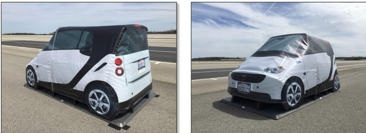
**Figure 9. Dynamic Research Inc. Guided Soft Target (GST). The surrogate vehicle is shown on top of the low profile robotic vehicle (LPRV) platform.**
