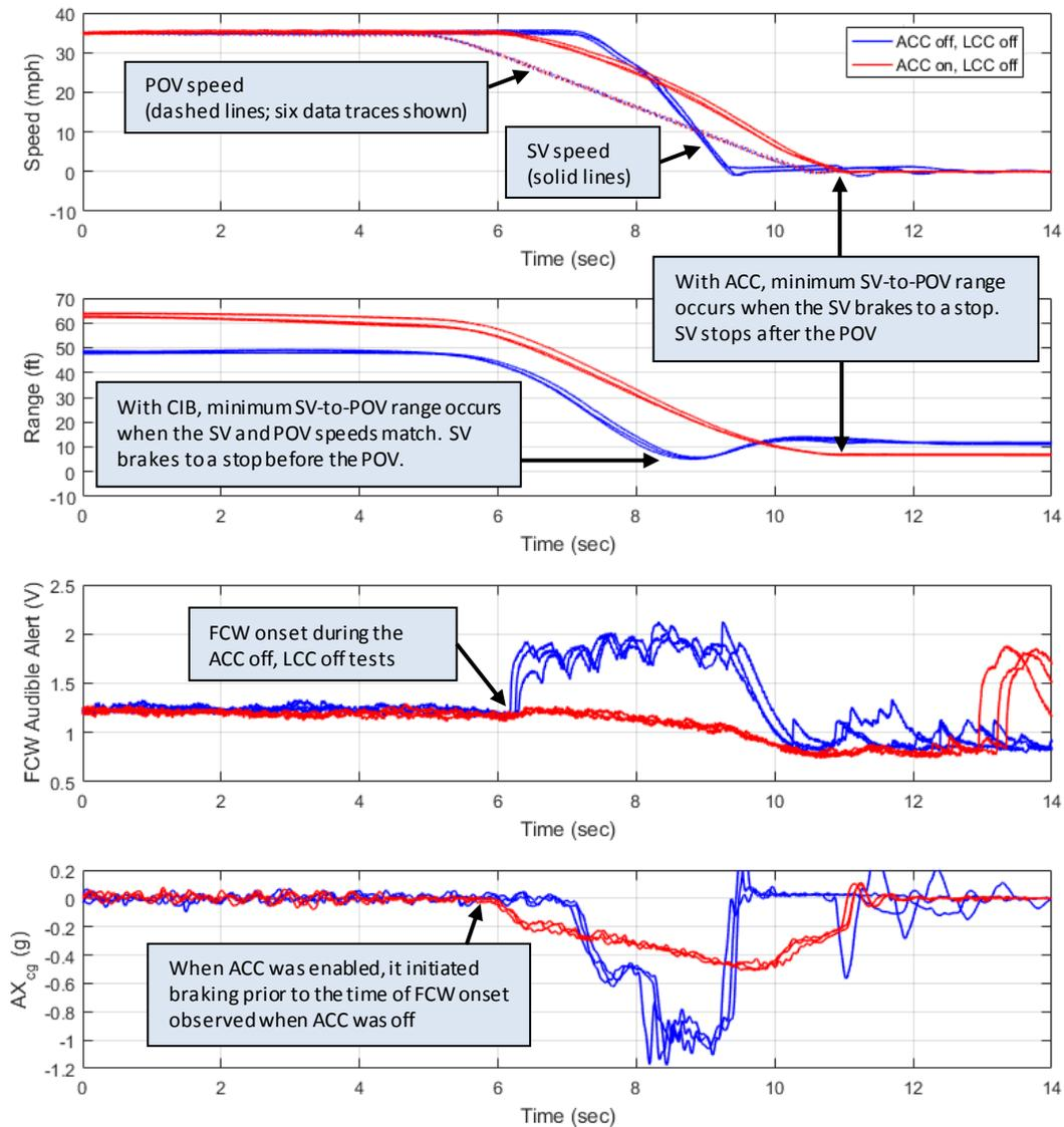
Figure 10. Mercedes C300 LVD\_35\_35 tests performed with ACC on and off.
