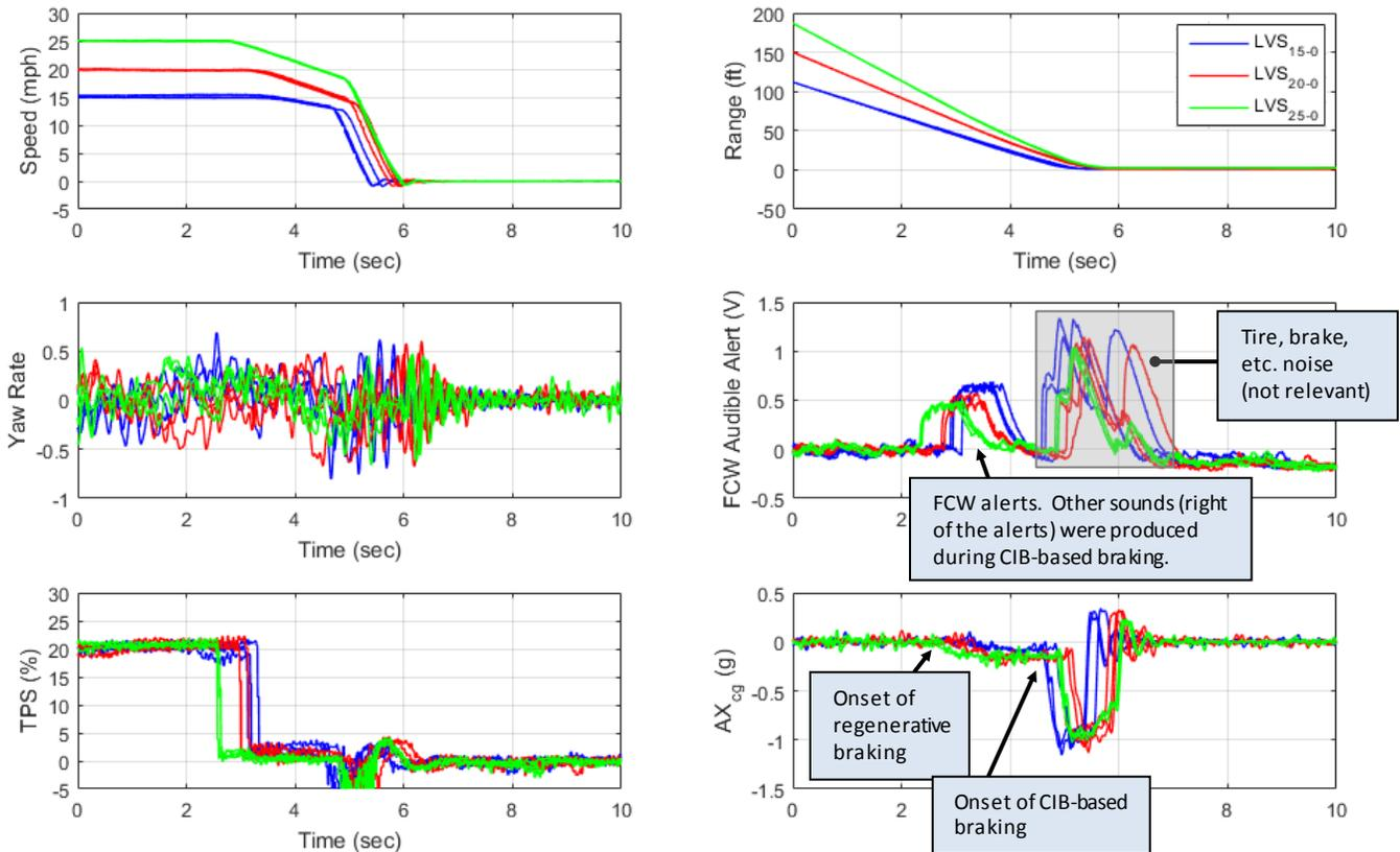
Figure 18. LVS tests performed with the Tesla Model S.
