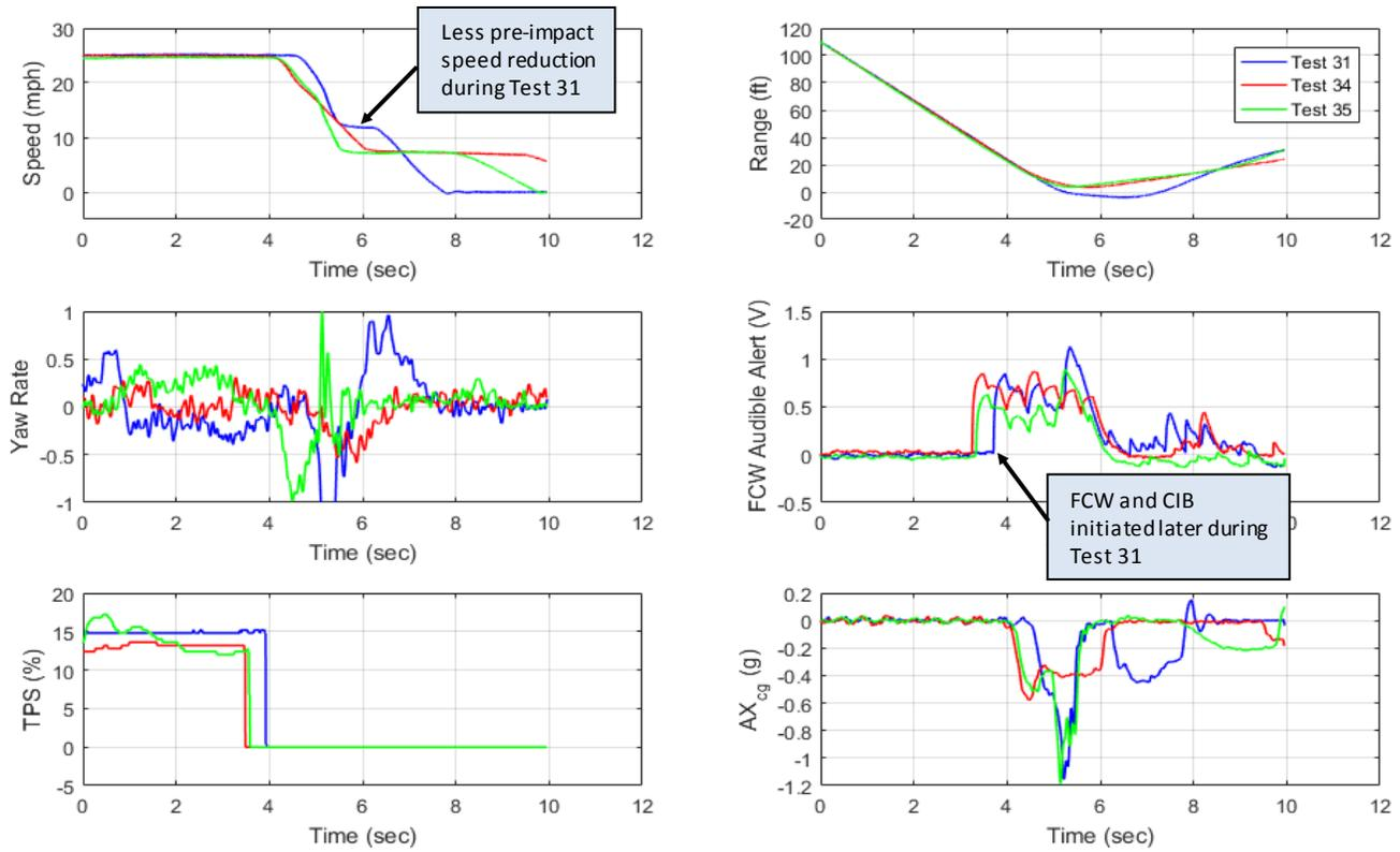
Figure 16. Mercedes C300 LVM\_25\_10 tests performed with no ACC or LCC.
