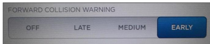
Figure 1. Tesla Model S forward collision warning settings. The “early” setting was selected for all tests described in this report.
