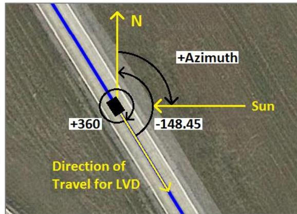
Figure A-2. Coordinate transformations used for LVM and LVD tests performed on the TRC Skid Pad.
