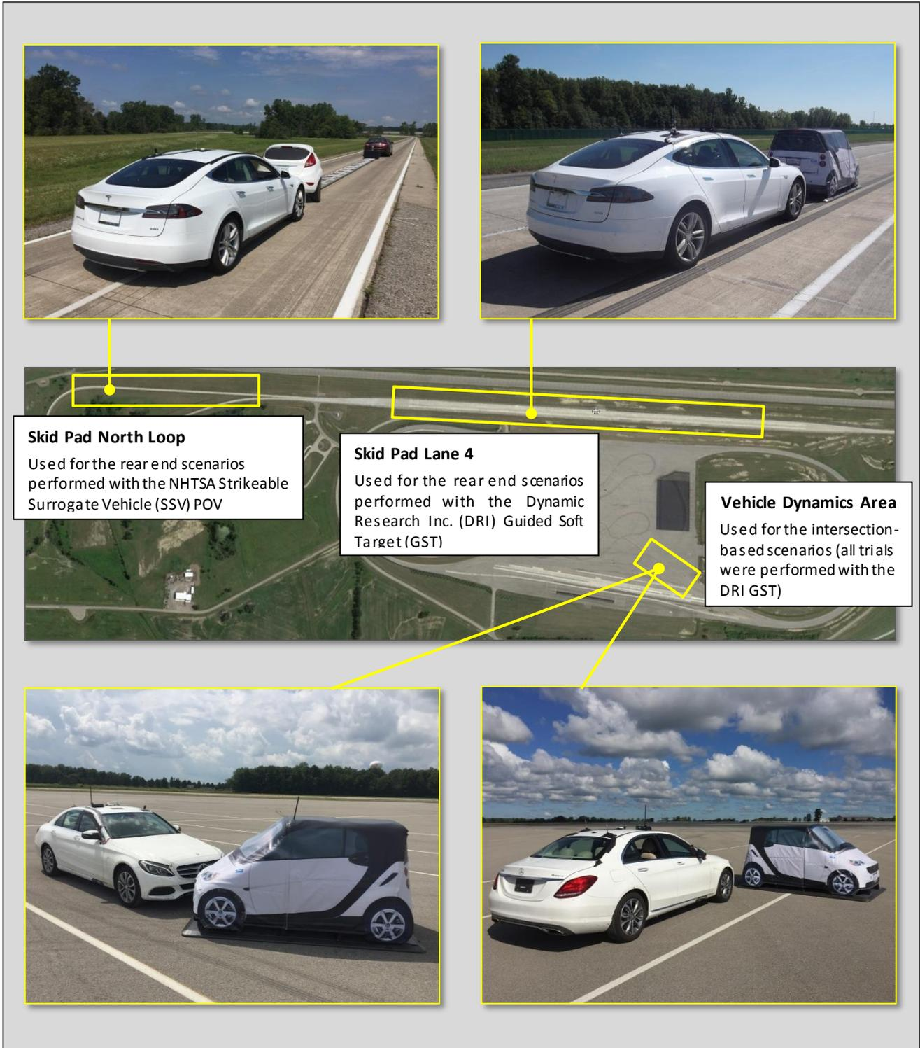
Figure 7. Test track facilities used for the scenarios described in this report.
