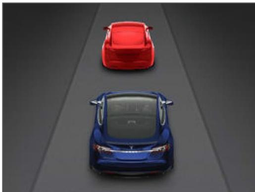
Figure 2. Tesla Model S visual FCW alert (as shown in the Tesla Model S operator's manual [2])
