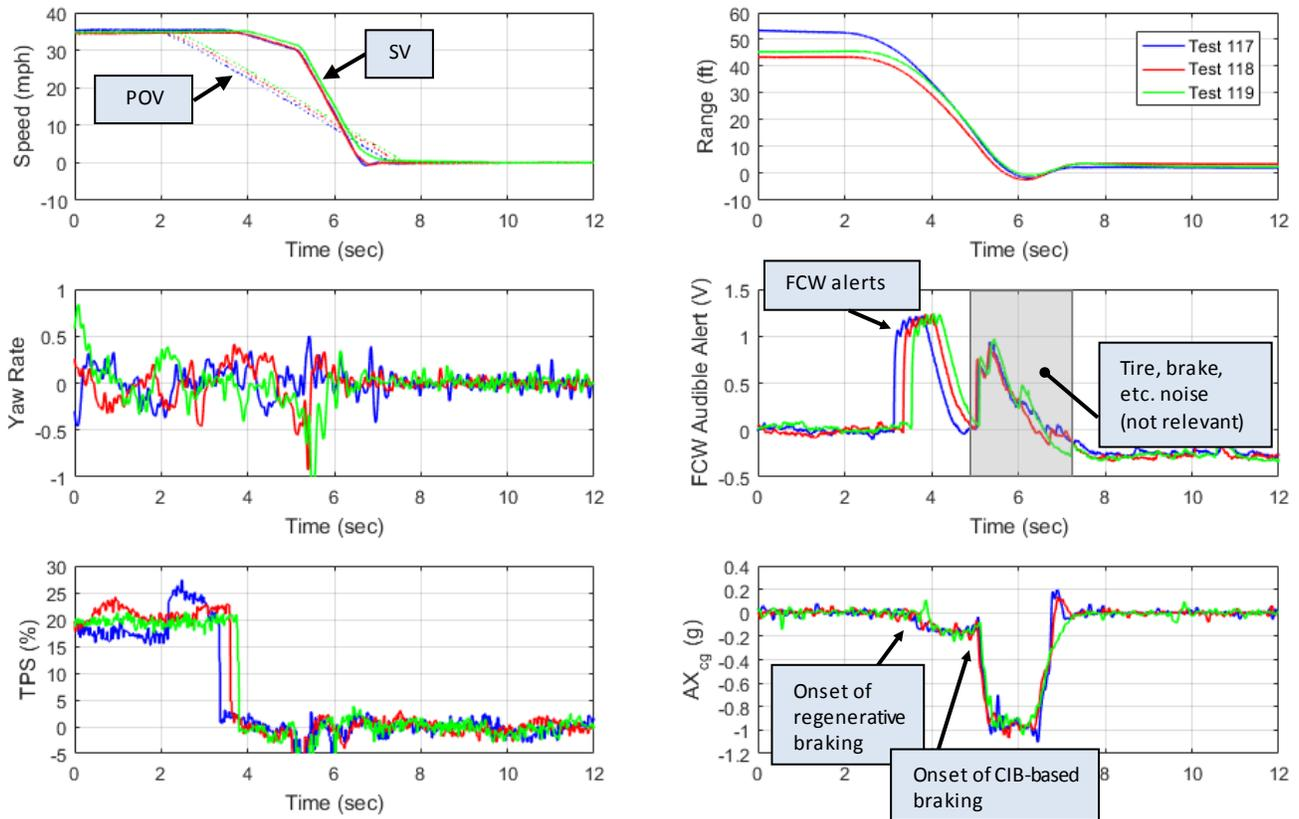
Figure 23. LVD\_35\_35 tests performed with the Tesla Model S.
