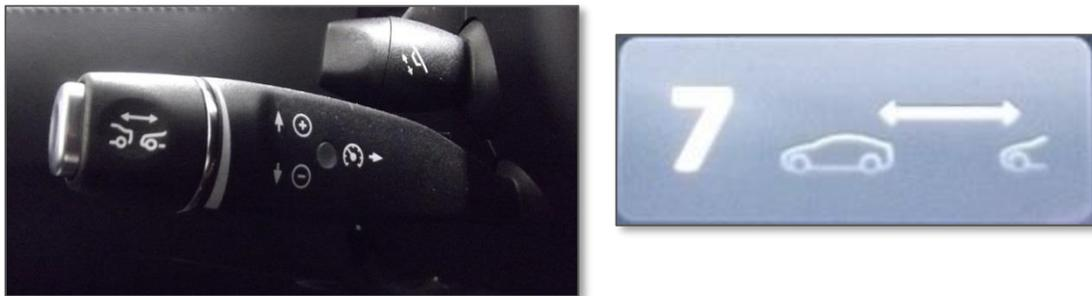
Figure 4. Tesla Model S adaptive cruise control and Autopilot stalk (left) and the corresponding proximity indication (right; presented on the left side of the vehicle's instrument cluster).
