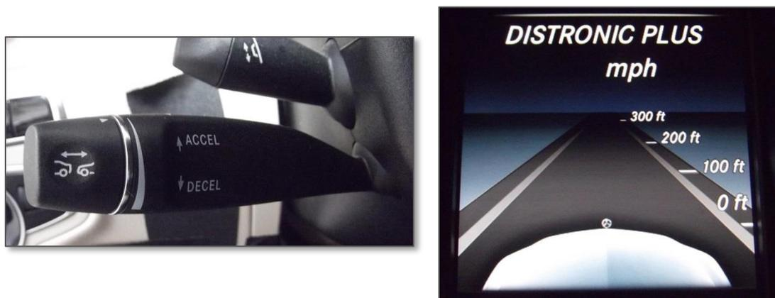
Figure 5. Mercedes C300 adaptive cruise control stalk (left) and the corresponding proximity indication (right; presented in the center of the vehicle's instrument cluster).
