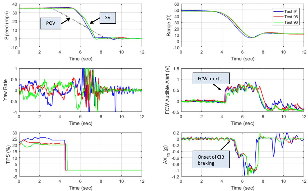
Figure 27. LVD\_35\_35 tests performed with the Mercedes C300.
