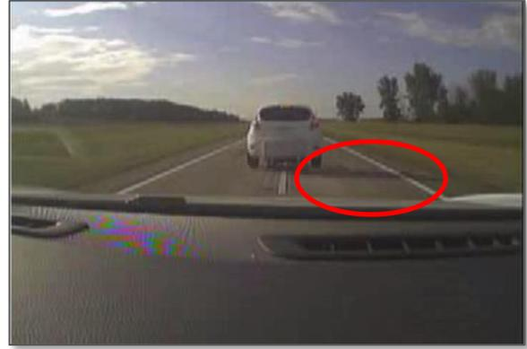
**Figure 31.** 25\_25 LVD Test 106 performed with the Tesla Model S. Note the presence of a shadow on the passenger side of the surrogate vehicle.
