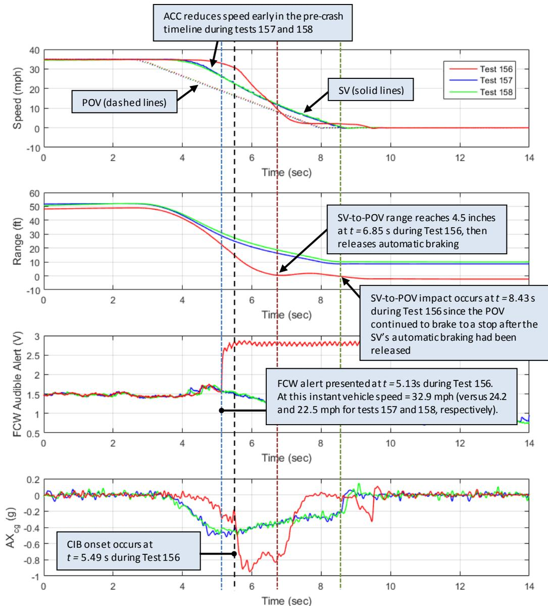
Figure 15. Tesla Model S LVD\_35\_35 tests performed with ACC and LCC enabled.
