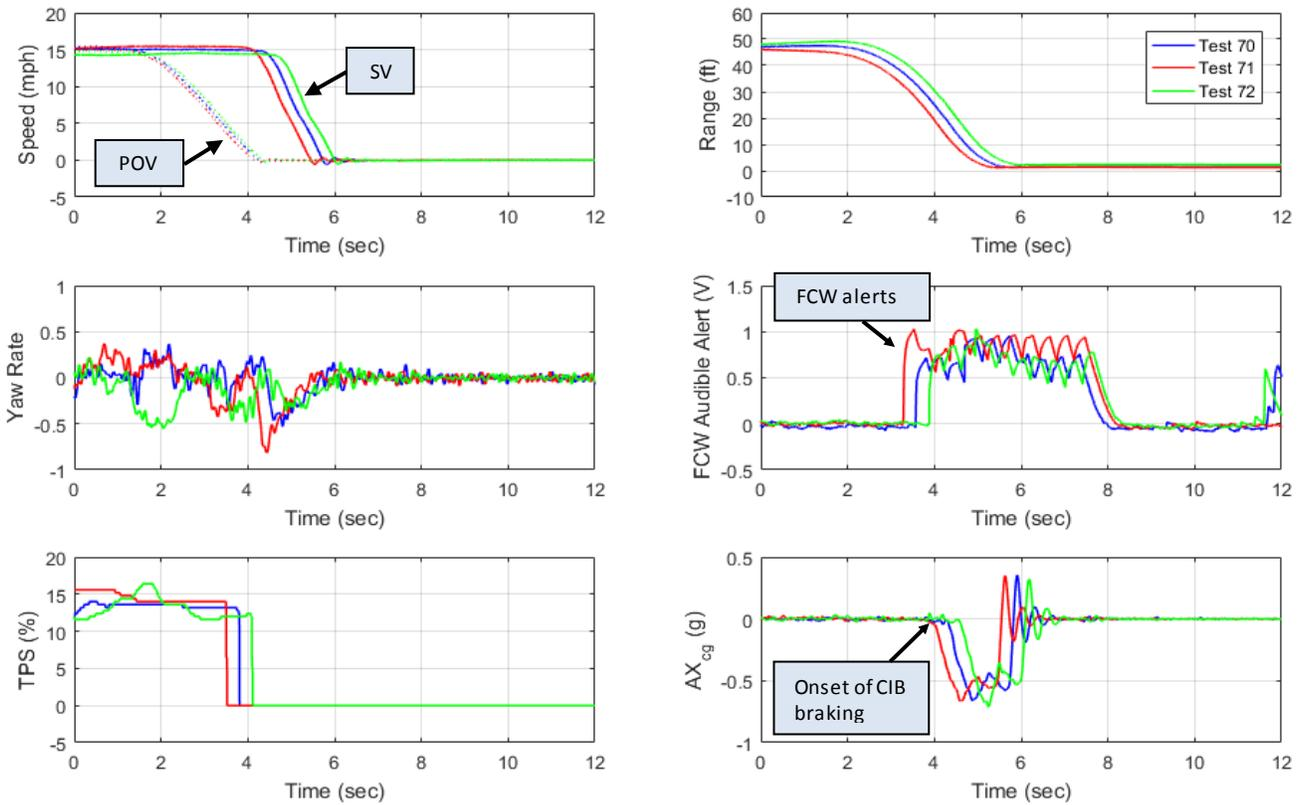
Figure 26. LVD\_15\_15 tests performed with the Mercedes C300.
