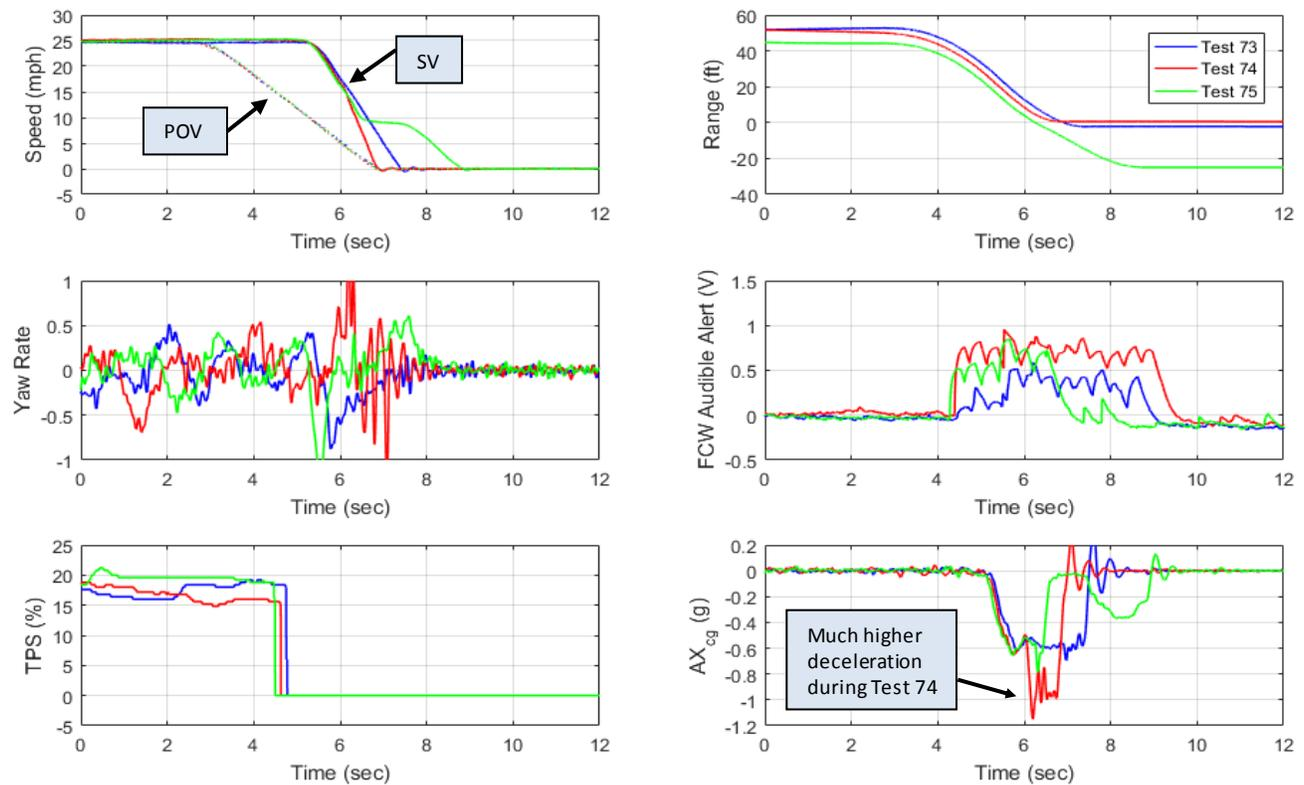
Figure 17. Mercedes C300 LVD\_25\_25 tests performed with no ACC or LCC.
