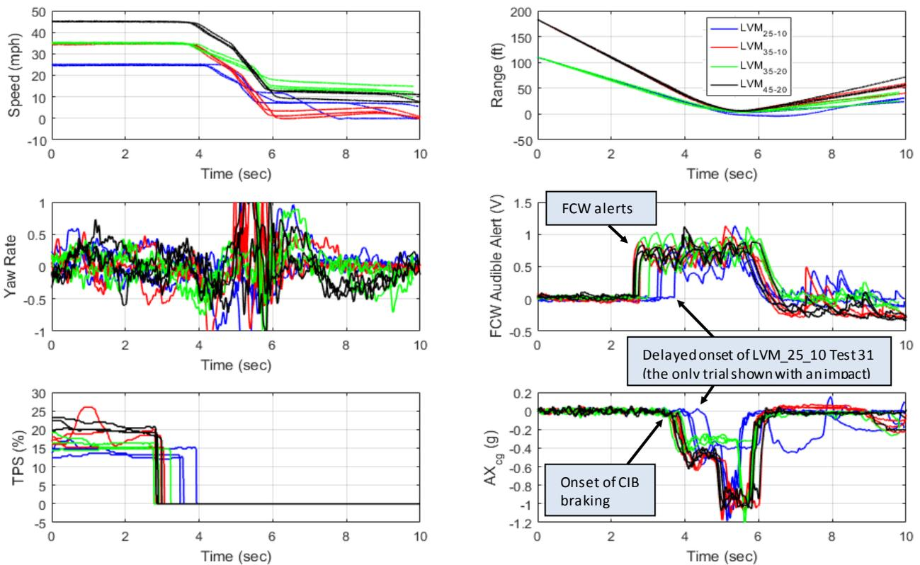
Figure 25. LVM tests performed with the Mercedes C300.
