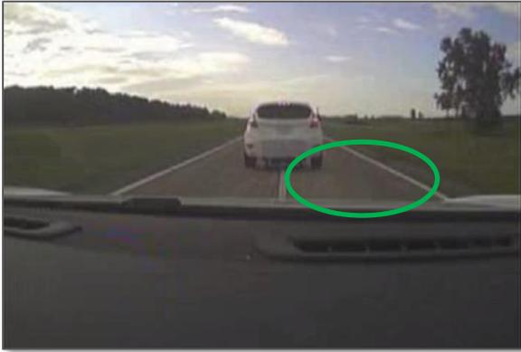
**Figure 30.** 25\_25 LVD Test 105 performed with the Tesla Model S. Note the absence of a shadow on the passenger side of the surrogate vehicle.
