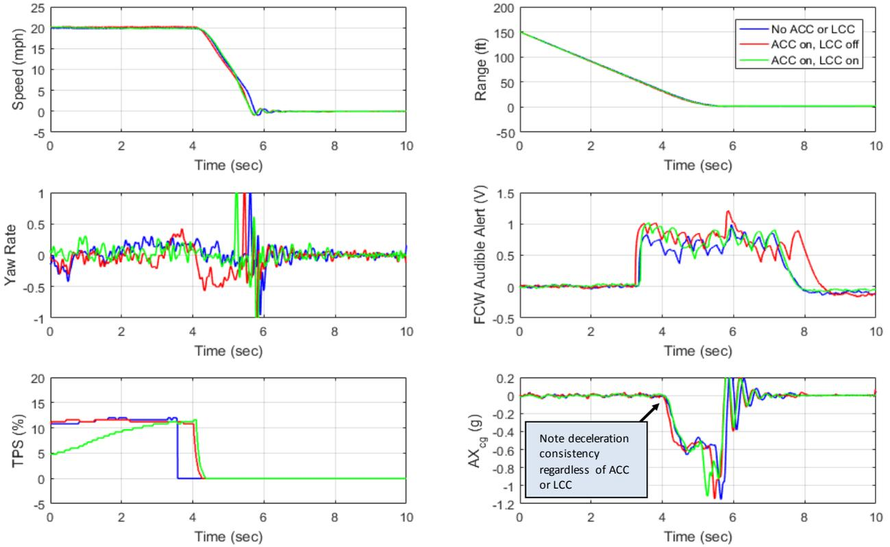
Figure 28. LVS\_20\_0 tests performed with the Mercedes C300.
