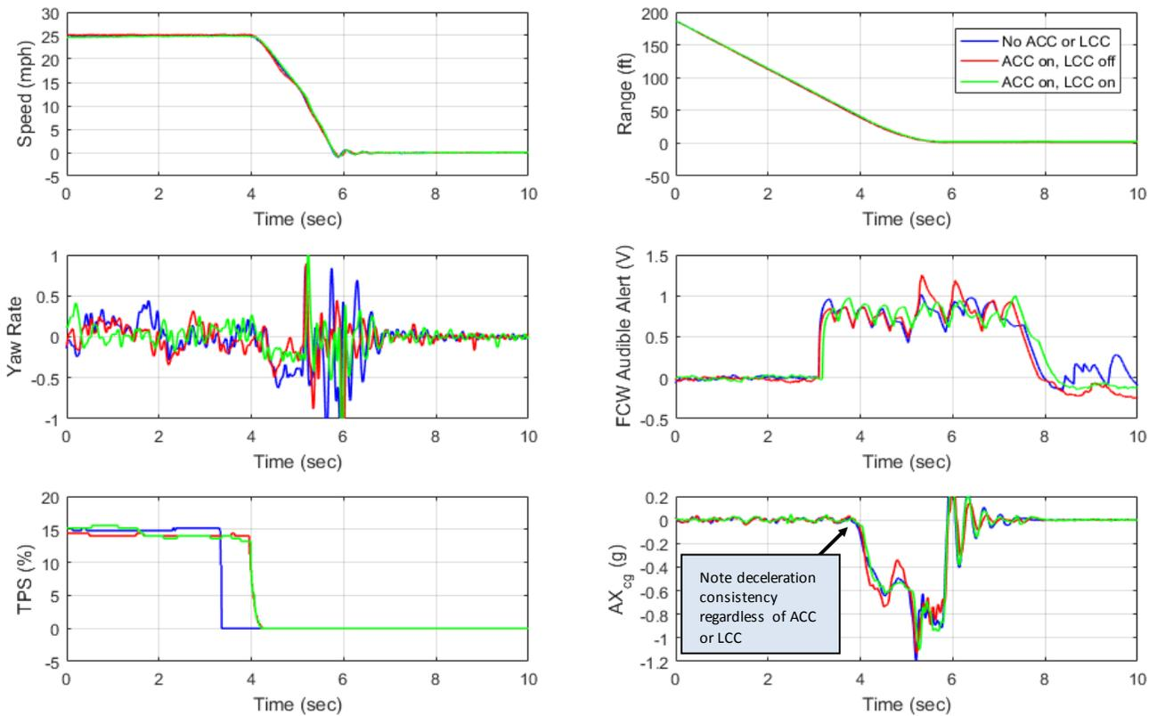
Figure 29. LVS\_25\_0 tests performed with the Mercedes C300.
