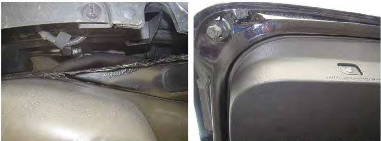
Figure 3. Underbody seam sealant and liftgate valve applied per TSB 14-0130 to 2014 Ford Explorer 3986.
