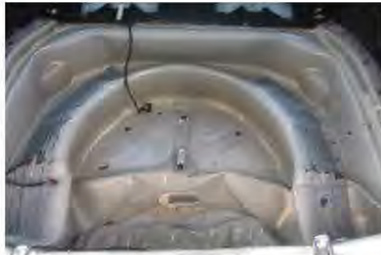
Figure 5 Photograph (SKZ3-000784) showing buckling of the rear floor pan area, where the spare tire resides.
