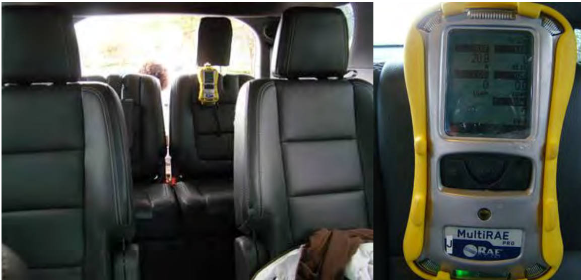
Figure 5. Gas monitor mounted under third row driver side headrest on 2014 Ford Explorer [REDACTED]. The calibration check mark is shown at right.
