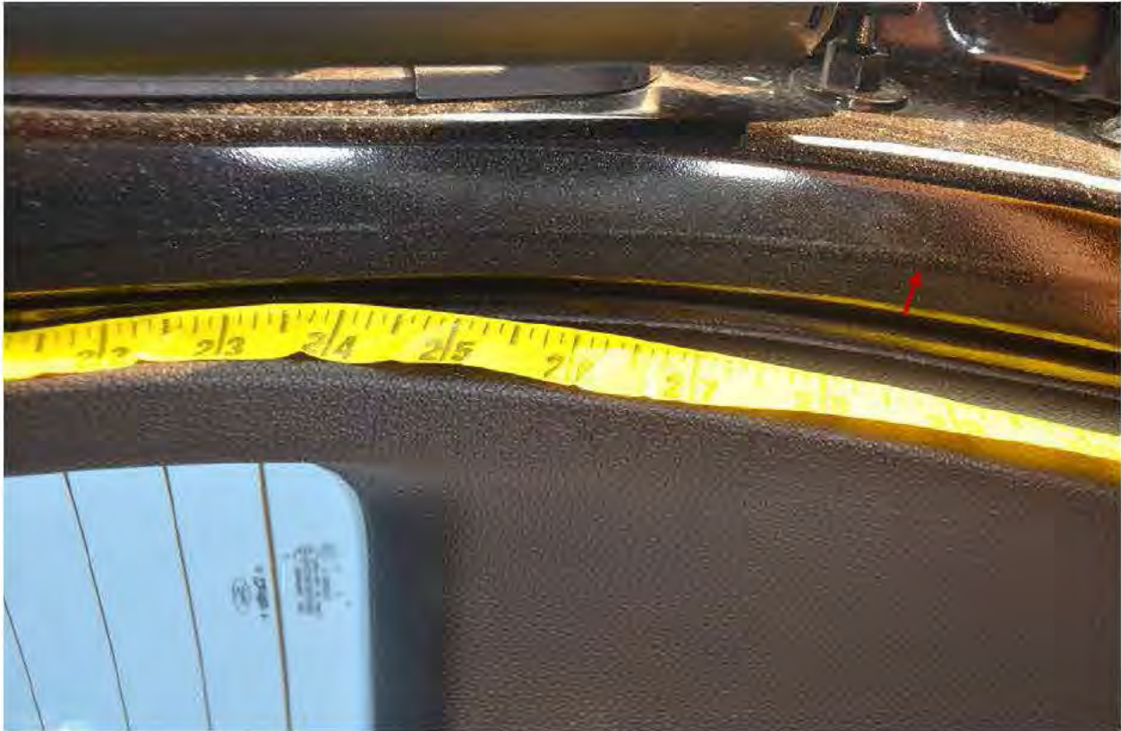
Figure 7 Photograph showing the witness marks on the repurchased vehicle. The witness marks appeared to be continuous along the perimeter of the hatch, with the exception of a small 0.1"-0.2" gap near the bottom.
