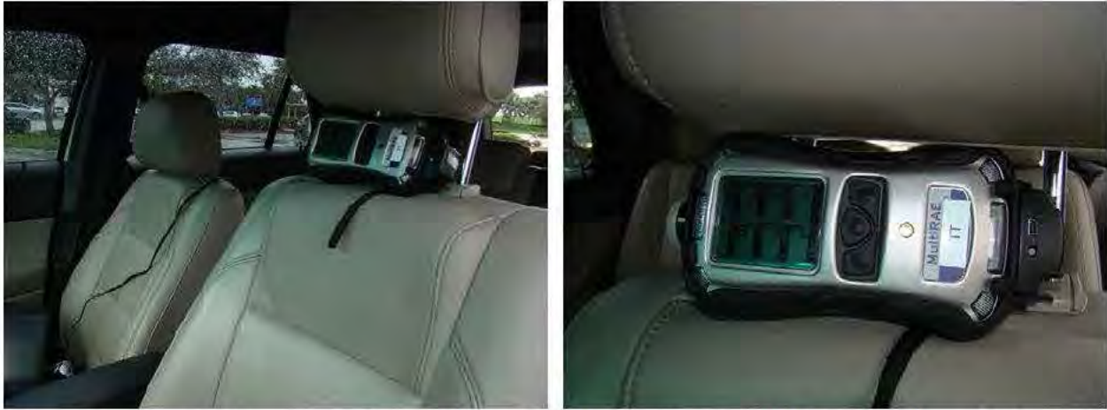
Figure 9. Gas monitor mounted under driver headrest on Dixon 2013 Ford Explorer 1363. The calibration check mark is shown at right.
