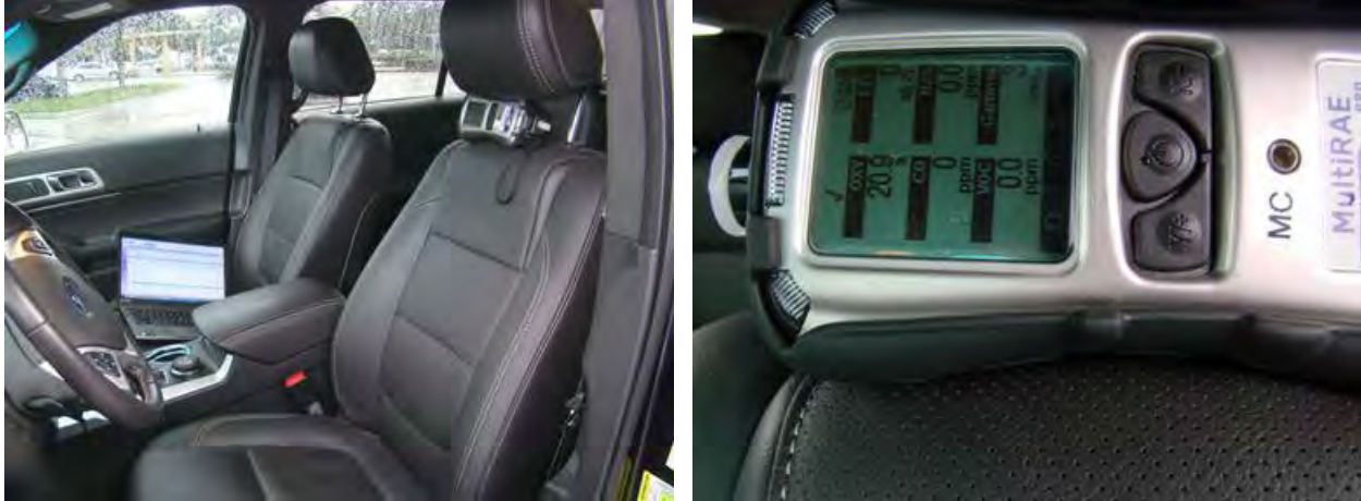
Figure 4. Gas monitor mounted under driver headrest on 2014 Ford Explorer [REDACTED]. The calibration check mark is shown at right.
