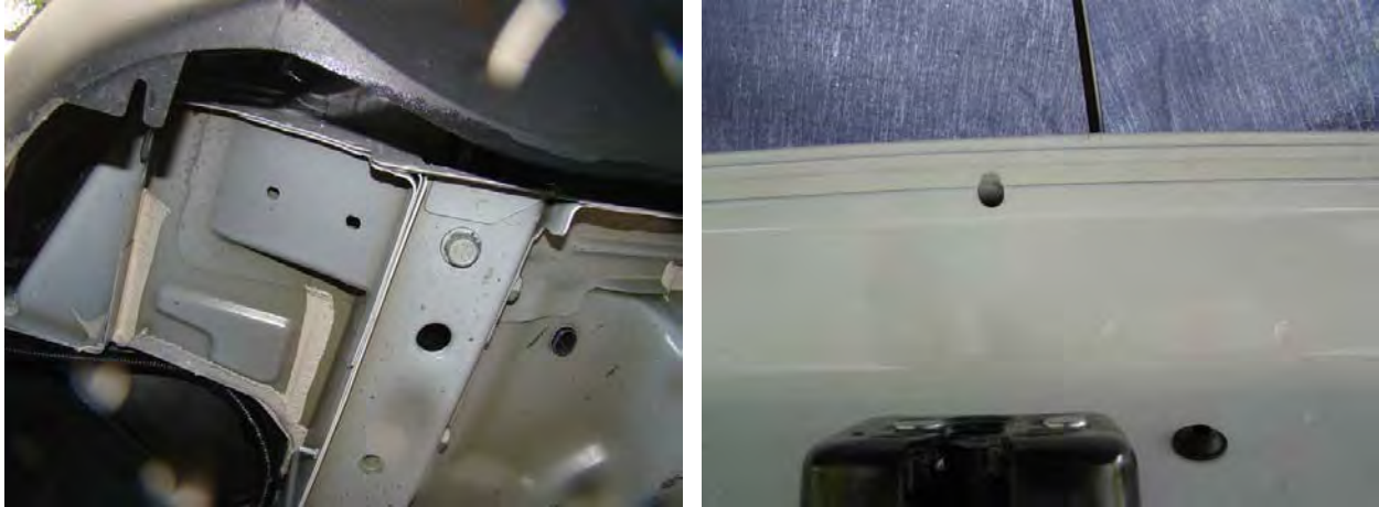
Figure 28. 2015 Jeep Grand Cherokee [REDACTED]. Intermittent underbody sealant at left. Open drain holes on the left, middle, and right sides at the latch end of the liftgate (top of photo).
