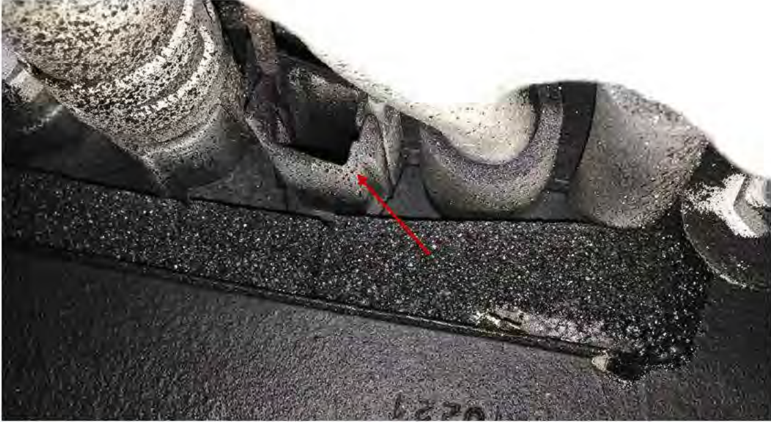
Figure 12 Photograph of the underbody of the Subject Vehicle showing the auxiliary climate control drain with 3M Rubberized Undercoating on it.
