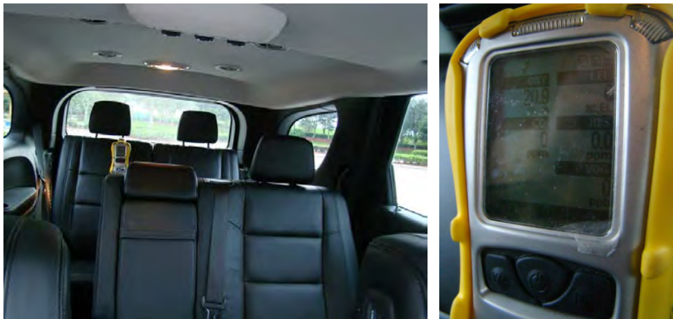
Figure 15. Gas monitor mounted under third row driver side headrest on 2015 Dodge Durango [REDACTED]. The calibration check mark is shown at right.
