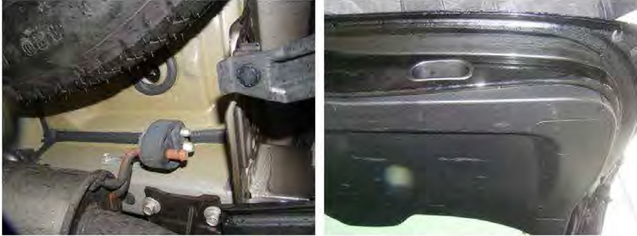
Figure 35. 2014 Toyota Highlander 6397. Underbody sealant at left. Outer drain holes are plugged on the left and right sides at the latch end of the liftgate. Middle hole is open (top of photo).
