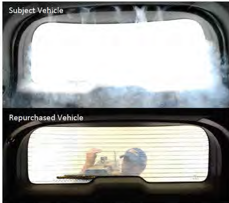
Figure 8 Screen captures taken approximately 30 seconds after the test was started in the Subject Vehicle (top) and in the repurchased vehicle (bottom).
