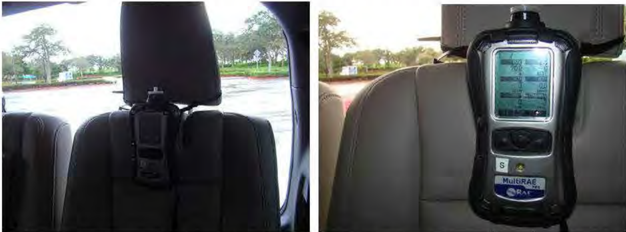
Figure 10. Gas monitor mounted under third row driver side headrest on [redacted] 2013 Ford Explorer [redacted]. The calibration check mark is shown at right.
