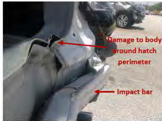
Figure 4 Photograph (SKZ3-000759) showing damage to the impact bar and the body at the hatch perimeter.
