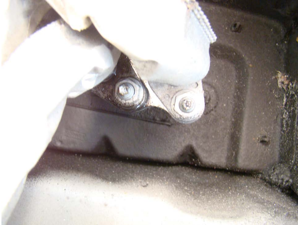
Figure 64: Photographs showing the underbody of the [REDACTED] vehicle. The sealer was not applied to all locations specified in the TSB.
