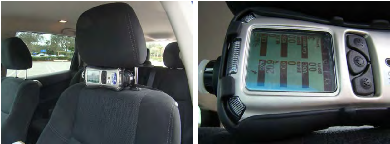
Figure 19. Gas monitor mounted under driver headrest on 2015 Nissan Pathfinder 0146. The calibration check mark is shown at right.
