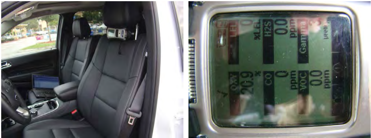
Figure 14. Gas monitor mounted under driver headrest on 2015 Dodge Durango [REDACTED]. The calibration check mark is shown at right.
