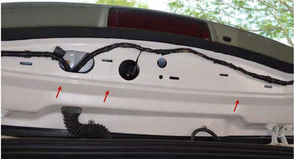
Figure 6 Witness marks from the seal on the top side of the rear hatch on the Subject Vehicle. Gaps are present.
