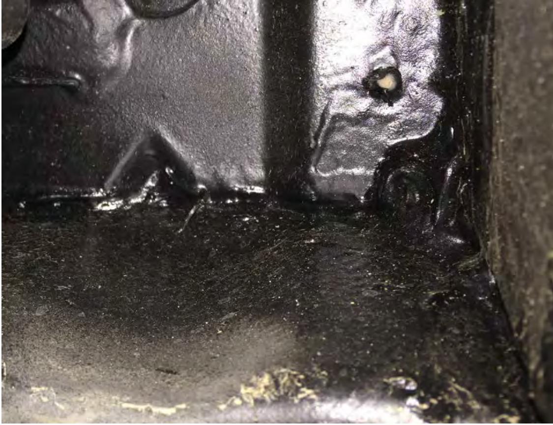
Figure 11 Photograph of the repurchased Explorer with the same field of view as in Figure 10 showing adequate application and coverage of the Motorcraft Seam Sealer and 3M Rubberized Undercoating.
