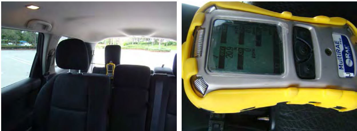
Figure 20. Gas monitor mounted under third row driver side headrest on 2015 Nissan Pathfinder 0146. The calibration check mark is shown at right.
