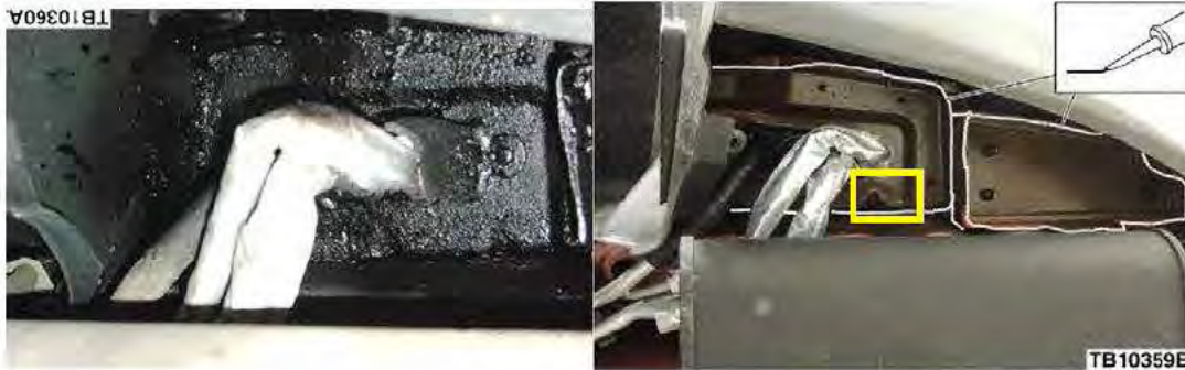
Figure 9 Photographs from TSB 12-12-4 illustrating areas on the driver’s side which are to be covered with a “generous” amount of 3M Rubberized Undercoating (left picture) and seams to seal with the Motorcraft Seam Sealer (right picture). The yellow box in the right picture shows the field of view for the picture of the Subject Vehicle in Figure 10 and repurchased Explorer in Figure 11.
