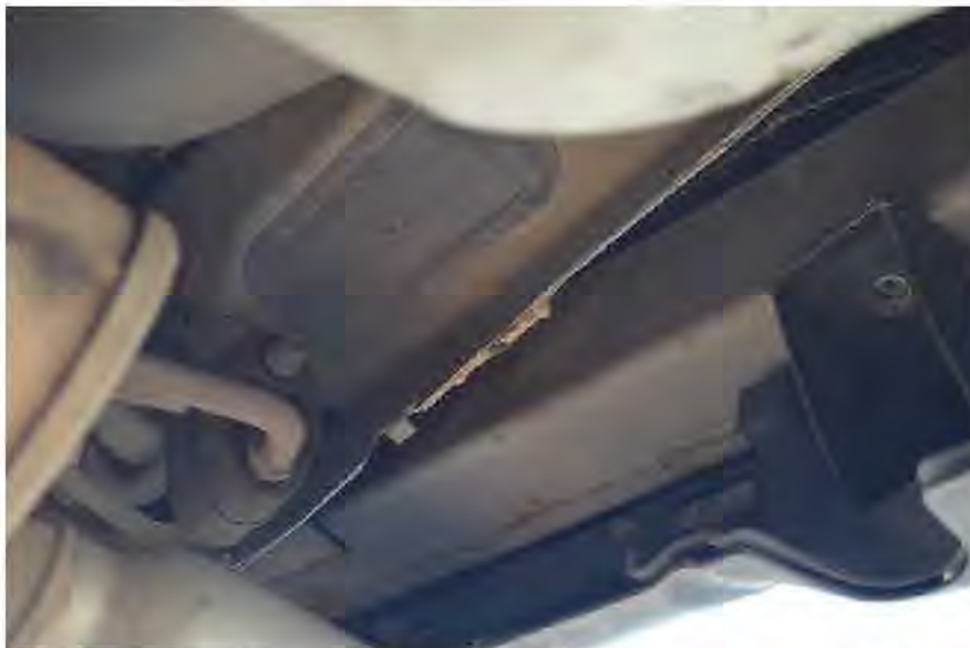
Figure 44. 2013 Ford Explorer [REDACTED] lack of underbody sealing.
