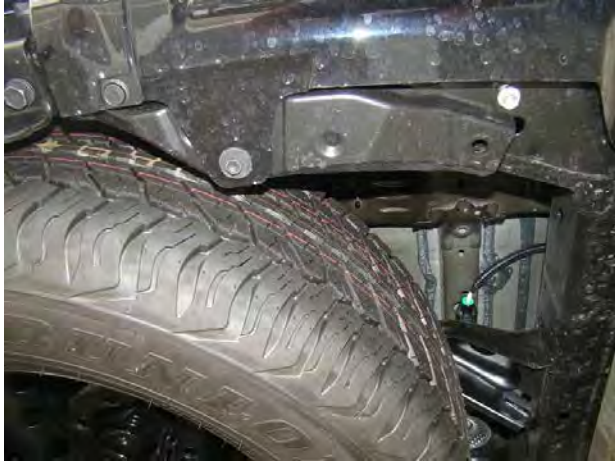
Figure 23. 2016 Toyota 4Runner [REDACTED]. Underbody sealant at left. Plugged drain holes on the left, middle, and right sides at the latch end of the liftgate (top of photo).
