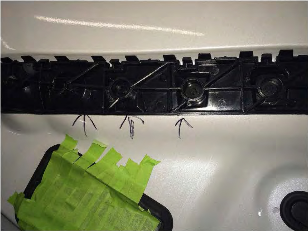
Leak under plastic bar that holds the bumper
