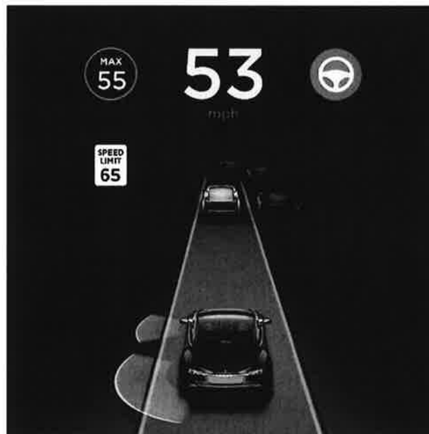
Figure 9. Autopilot user interface showing vehicle-perceived lane lines, other vehicles, and ultrasonic objects
