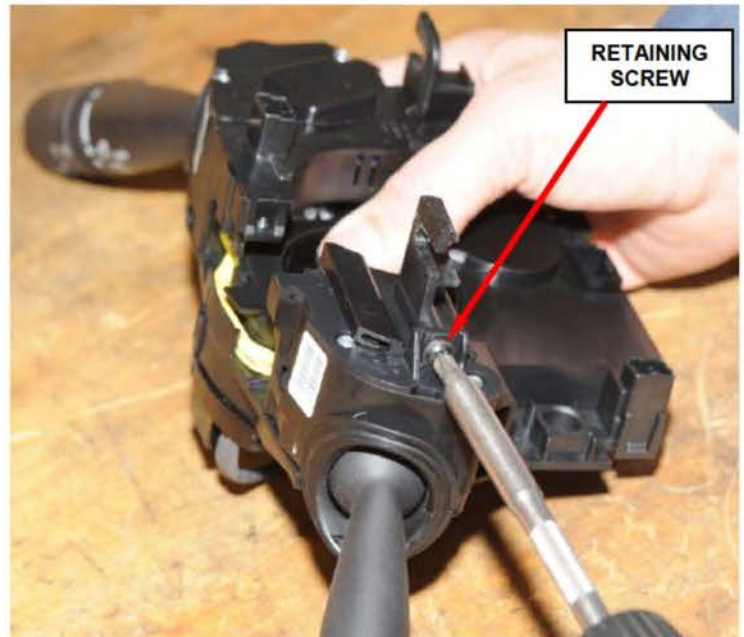
Figure 5 – Right Multi-Function Switch Retaining Screw
