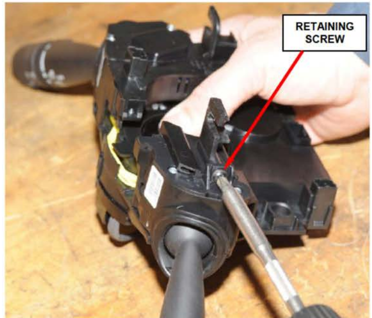
Figure 5 – Right Multi-Function Switch Retaining Screw
