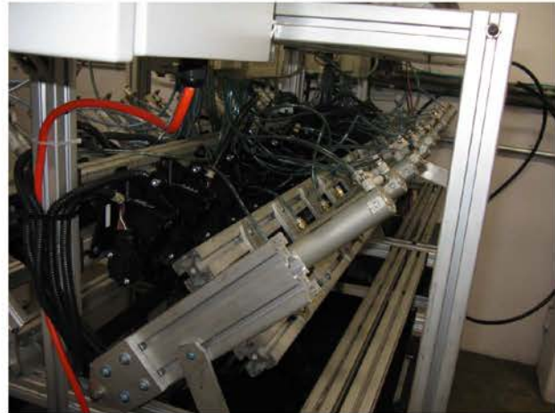
Figure 6—400483 UUT 17-30 on high speed cycle test fixture
