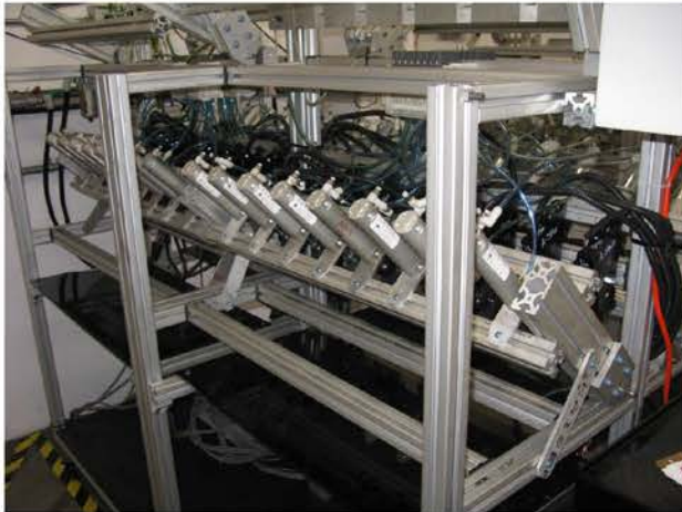
Figure 5—400483 UUT 01-16 on high speed cycle test fixture
