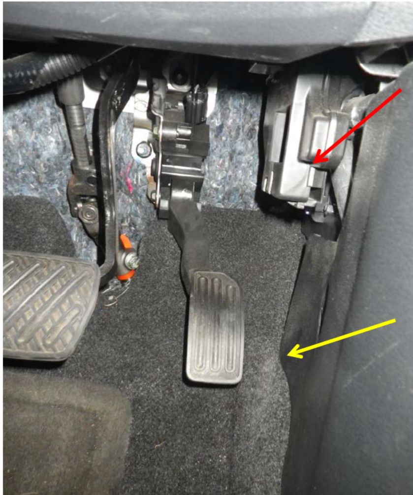
Figure 3. Position of HVAC actuator, red arrow, and trim panel corner, yellow arrow.
