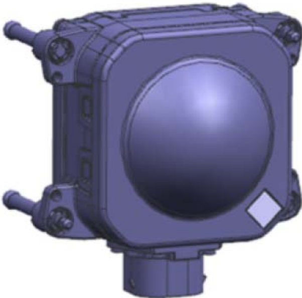
Figure 1. Driver Assistance System Module (long-range radar).
