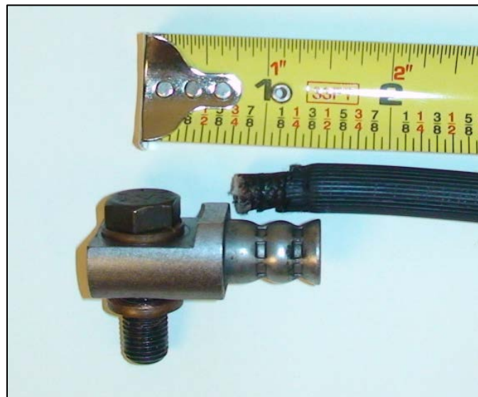
Figure 4. Sacramento EVOQ crimp failure mode.
