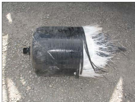
Figure 10: Displaced section of ruptured CNG cylinder
