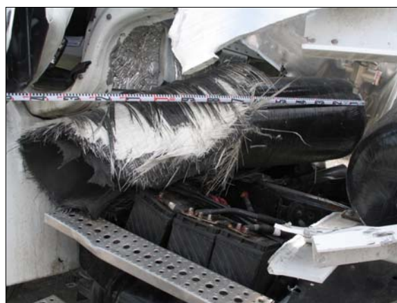
Figure 9: Ruptured CNG cylinder
