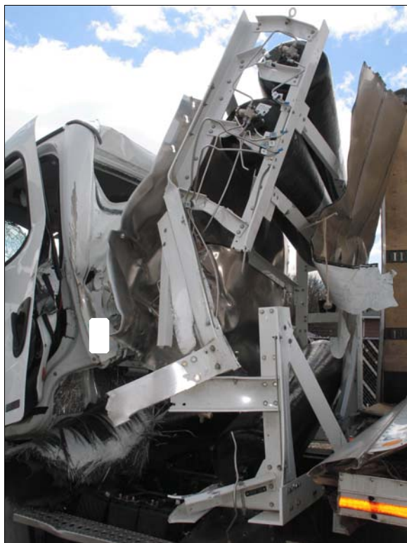
Figure 7: Left side damage to fuel cabinet
