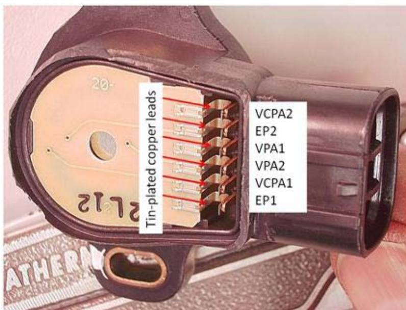
Figure 6.6.2.3-5. Disassembled Accelerator Pedal Assembly Potentiometer
