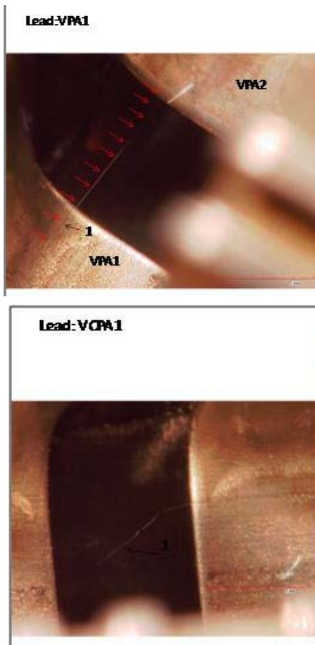
Figure 6.6.2.3-6. Shorting whisker VPA1 to VPA2 (top) and long whisker on VCPA1 (bottom)
