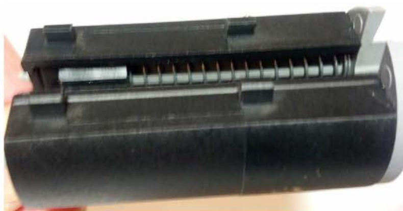
Figure 2 – Clutch Interlock Switch and View of a Return Spring
