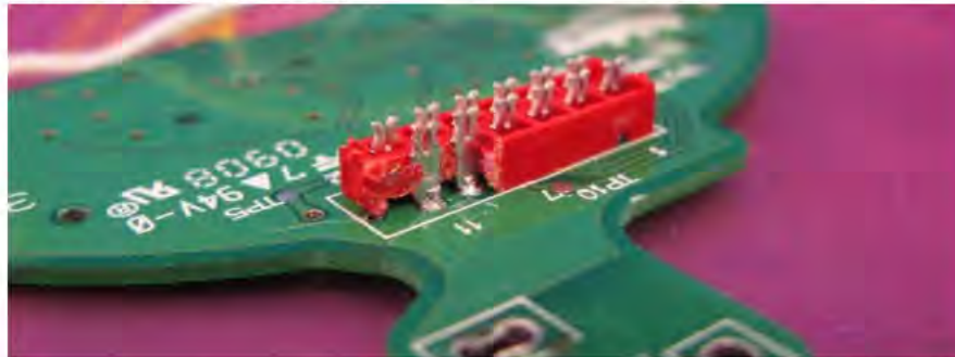
Motor PCB connect pin with sectioned to show pins
