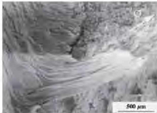
Fig. 11. SEM micrograph of a detail of a macrofibril within the coarse fibrillar zone.
