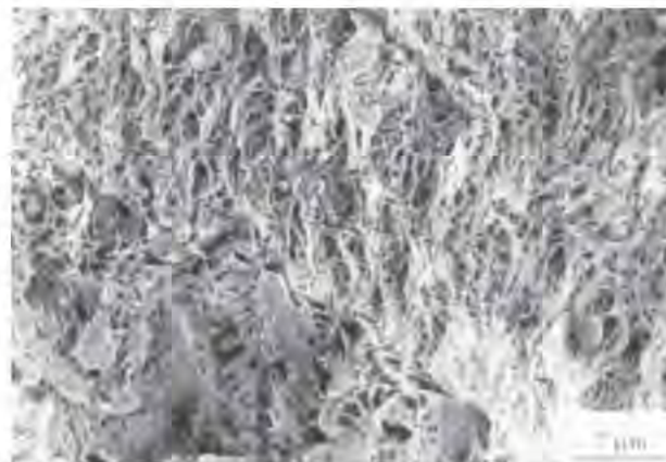
Fig. 13. SEM micrograph of a detail of the damage zone from a tensile fracture surface.
