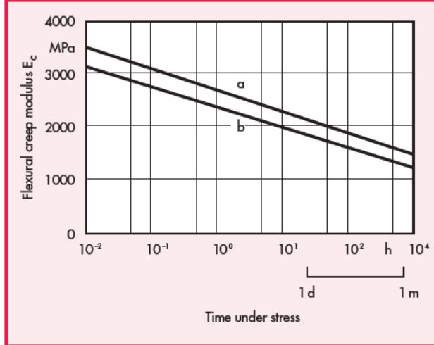
Fig. 9 · Flexural creep modulus of Hostaform C 13031 (a) and Hostaform C 13021 (b) (test specimen injection moulded, outer-fibre stress \sigma_b = 10 MPa, test temperature 23°C)
