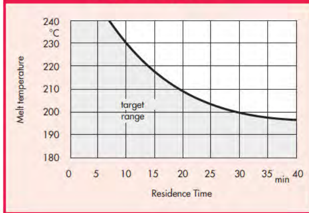
Fig. 42 · Recommended maximum residence time of Hostaform basic grades in the plasticizing cylinder of a processing machine
