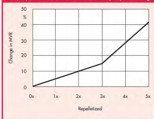
Fig. 92 · Change in the volume flow rate (MVR) of polyacetals as a function of multiple processing
