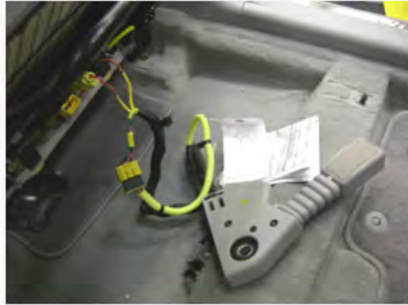
Incident seat belt buckles were test installed into a known good vehicle for evaluation
