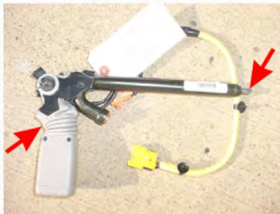
Seat belt buckle has already been deployed by the dealer before shipment to HMA
