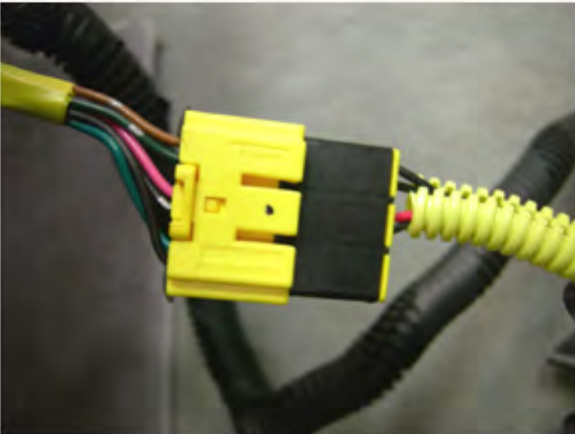
Seat belt buckle connector does not have a secondary latch
