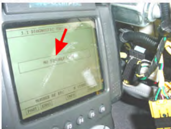
The seat belt buckle failure condition could not be duplicated when test installed in the vehicle
