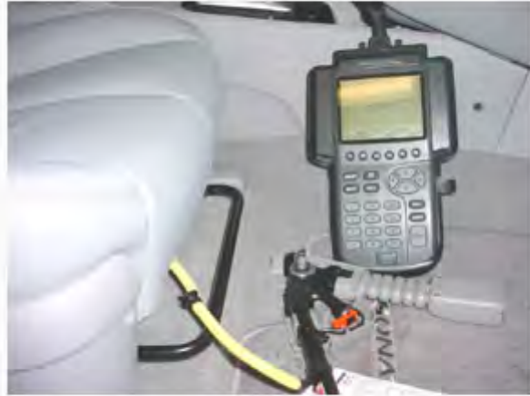
RH seat belt buckle assembly installed to known good vehicle for evaluation
