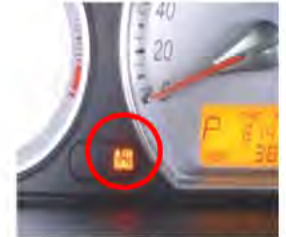
<A/bag warning light "ON">
