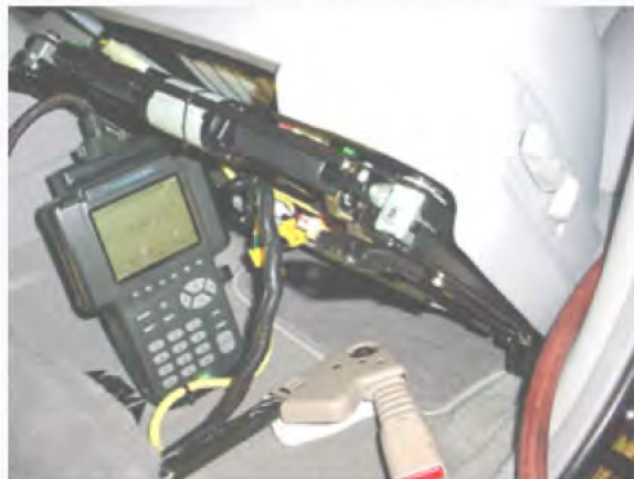
Incident LH seat belt buckles were test installed to a known "good" vehicle for evaluation
