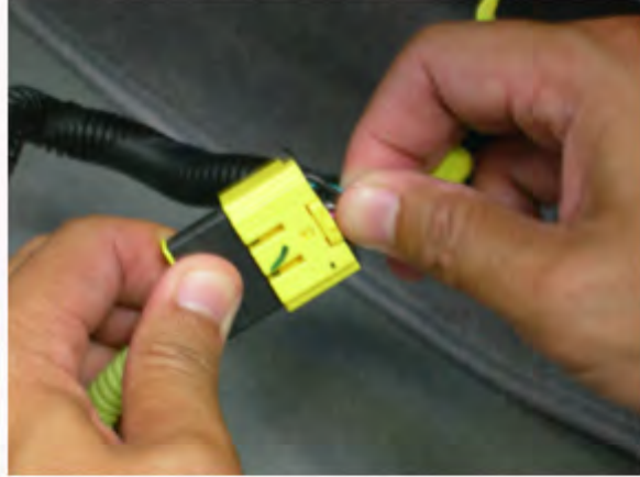
There was noticeable play when the seat belt connector was pulled in the closed position
