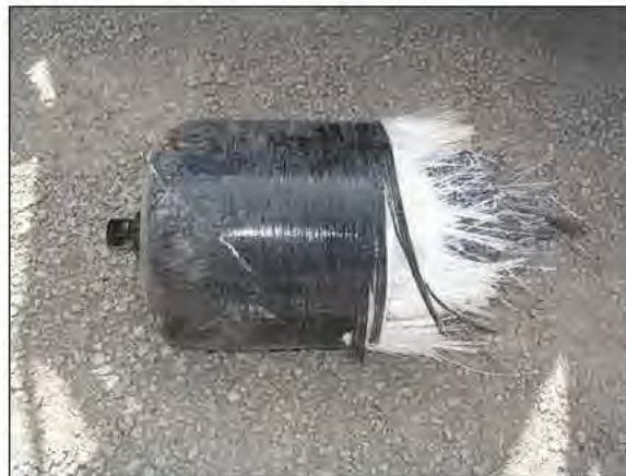
Figure 10: Displaced section of ruptured CNG cylinder
