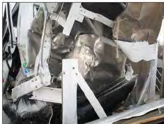
Figure 12: Exterior view of intrusion of back wall of Freightliner's cab
