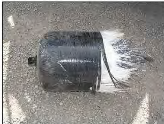
Figure 10: Displaced section of ruptured CNG cylinder
