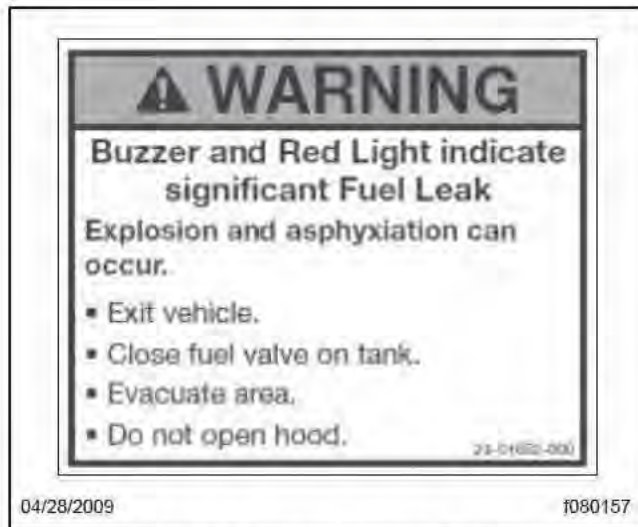
Fig. 16.4, Interior Warning Sticker
