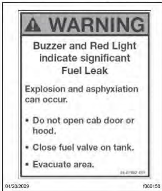
Fig. 16.5, Exterior Warning Sticker
