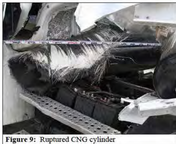
Figure 9: Ruptured CNG cylinder
