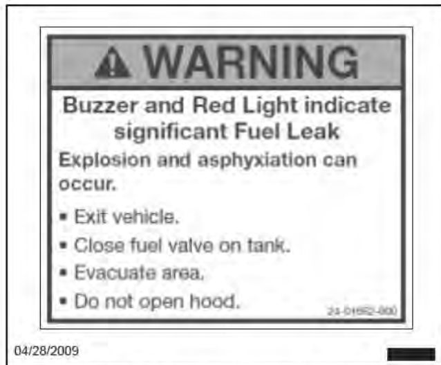
Fig. 16.4, Interior Warning Sticker
