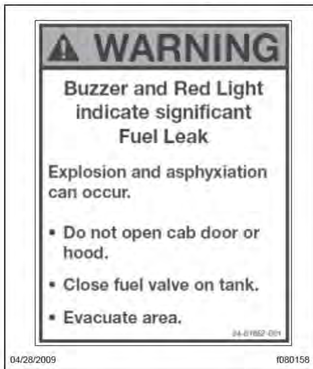
Fig. 16.5, Exterior Warning Sticker
