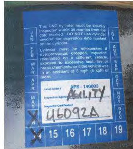
Fig. 2 A CNG cylinder inspection record label used to document completed inspections.
