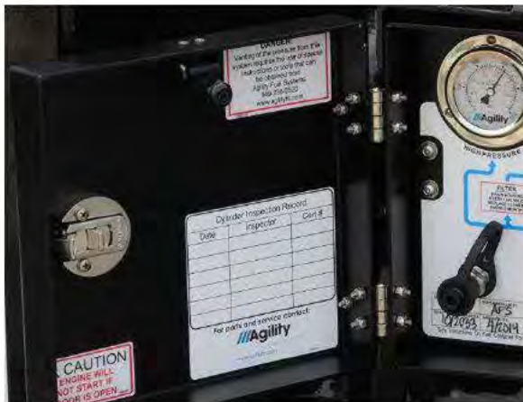
Fig. 3 An Agility Fuel Systems CNG cylinder inspection record decal (part number 10602107) on a fuel management module door.
