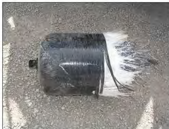
Figure 10: Displaced section of ruptured CNG cylinder
