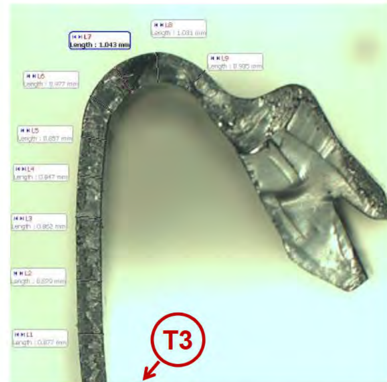
Sample HSM_F_06_271112 – New Tool (Rev F) Failed at 62,868 cycles (location T3)
