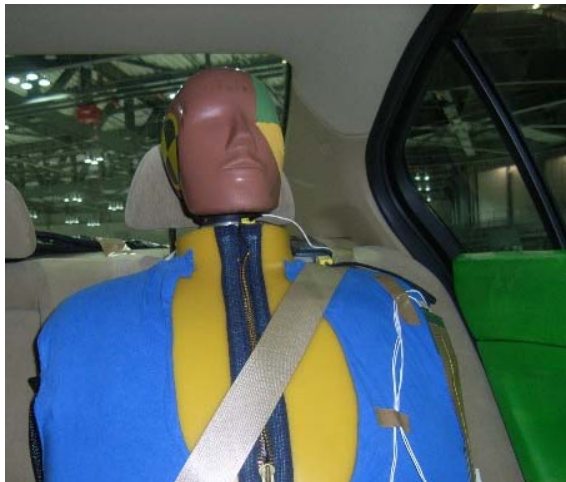
AM50% dummy seated aligned to the center of the seat.
