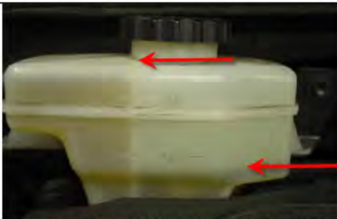
Condition of Brake Fluid in the Reservoir when DTC C1202 set
