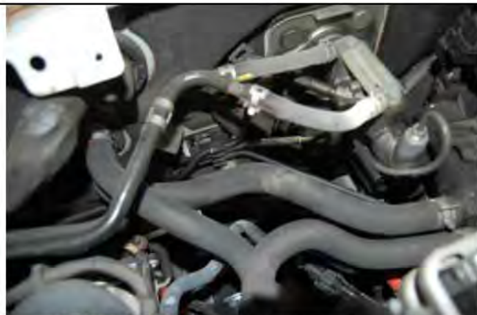
ABOVE / BELOW: Brake master cylinder fluid accumulation.
