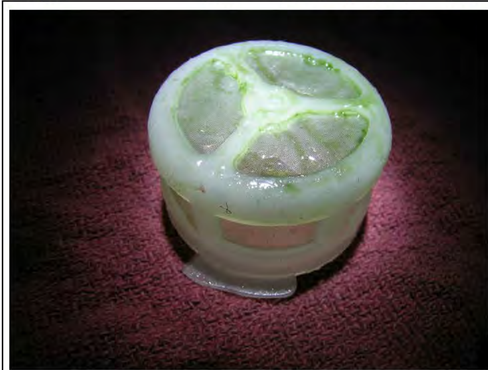
Bottom side of the brake reservoir fill hole filter showing the green substance deposited on the surface
