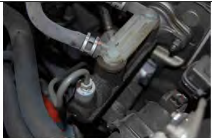
ABOVE: Brake master cylinder fluid accumulation. BELOW: : Stroke simulator area fluid accumulation.
