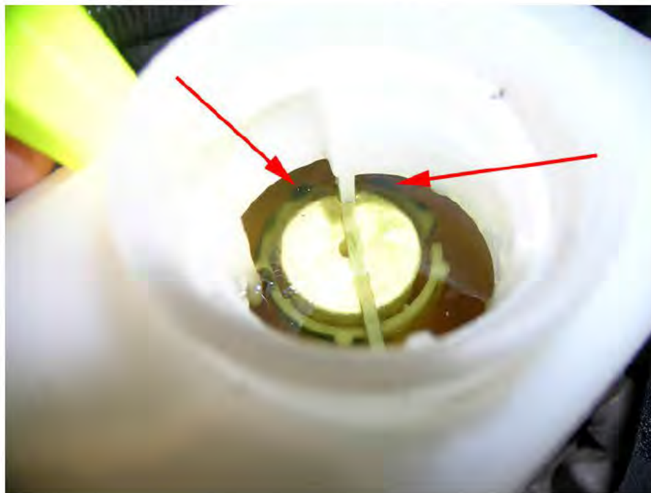
Green substance deposited on the inner surfaces of the brake reservoir
