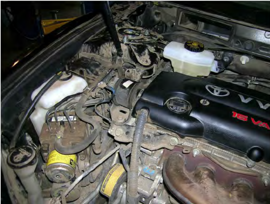
The reservoir was replaced with a new part and was filled with new brake fluid
