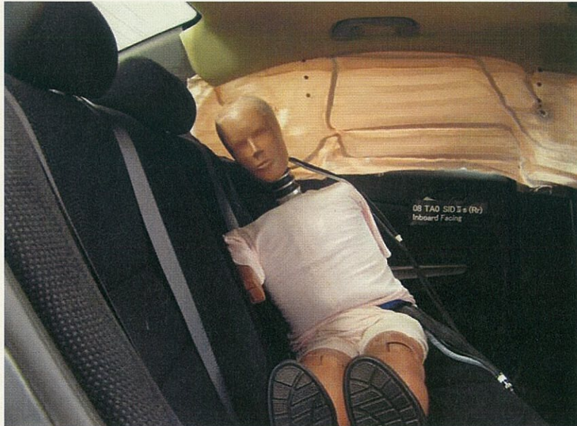
SID-IIs INBOARD FACING ON RAISED SEAT
