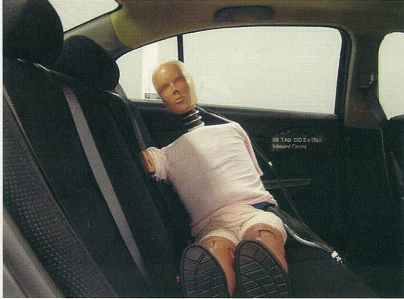
SID-IIs INBOARD FACING ON RAISED SEAT
