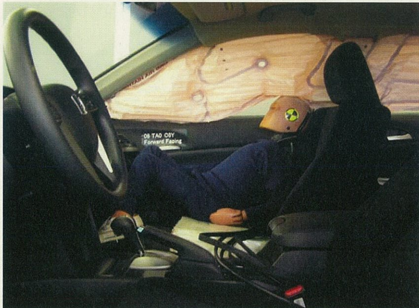
HYBRID III 6-YEAR-OLD CHILD DUMMY FORWARD FACING ON BOOSTER SEAT
