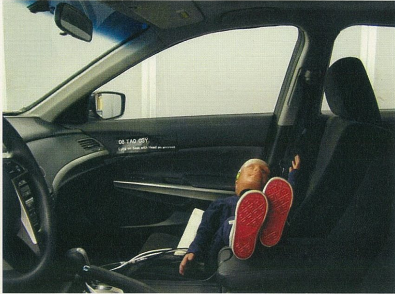
HYBRID III 3-YEAR-OLD CHILD DUMMY LYING ON SEAT, HEAD ON ARMREST
