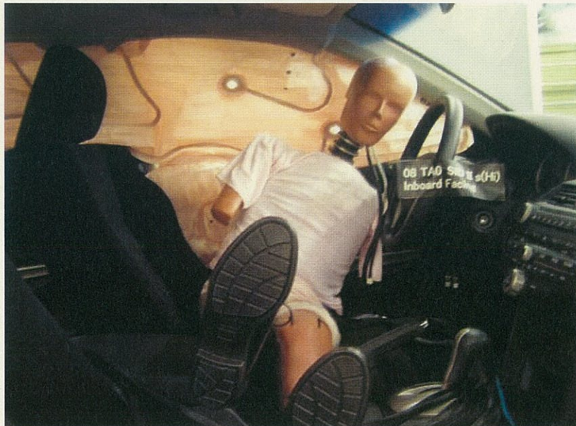
SID-IIs INBOARD FACING ON RAISED SEAT
