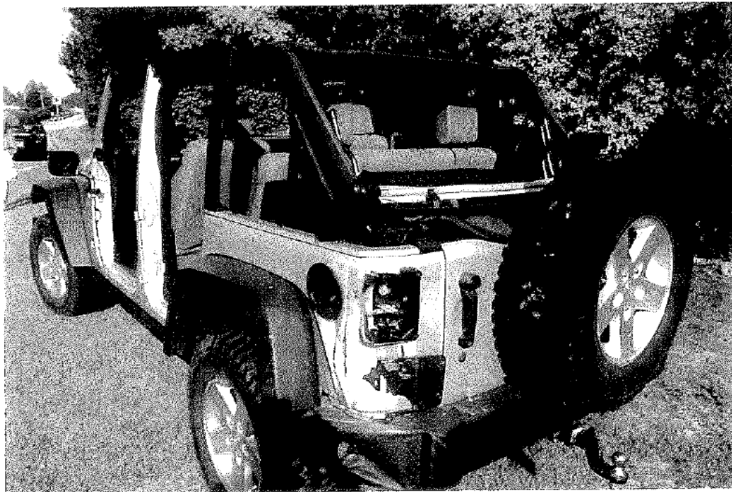
Figure 9: Damage to left rear tail light and bumper, vehicle #2, Jeep Wrangler.
