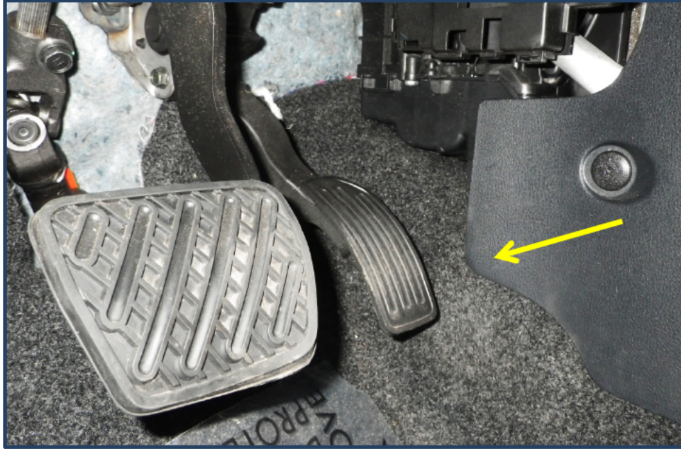
Figure 1: Position of trim panel MY 2013 Versa (Arrow indicates corner that interferes with driver's shoe)
