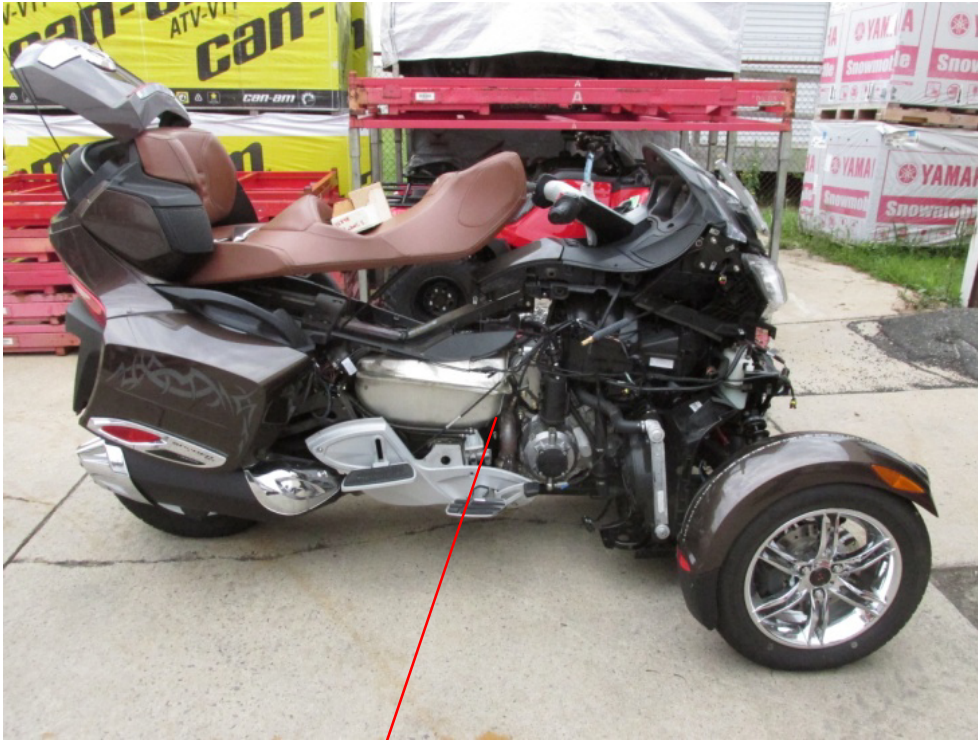
Figures 1-3 -- proximity of exhaust headers to fuel system.
