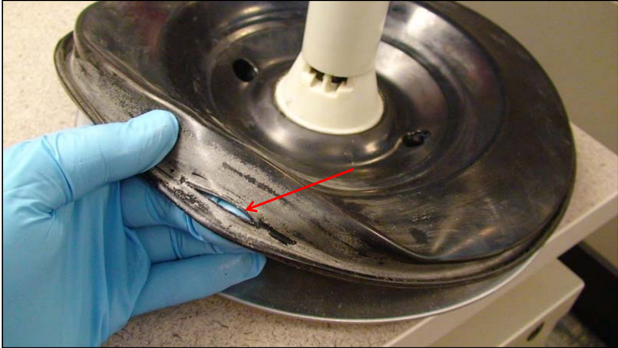
Figure 3. Diaphragm tear location (30 mm tear).
