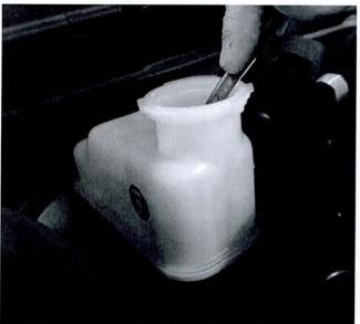
4. Fill the reservoir to the MAX line using DOT4 brake fluid.
