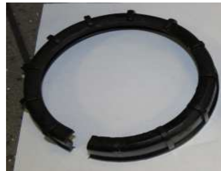
Broken ring nut, probably resulting from over-torquing
