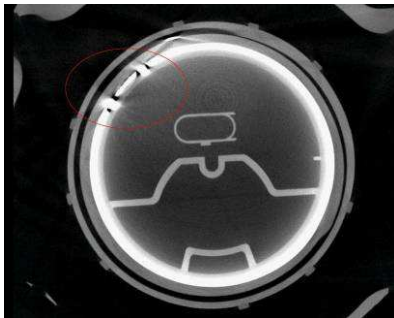
Pinched wires (CT)
