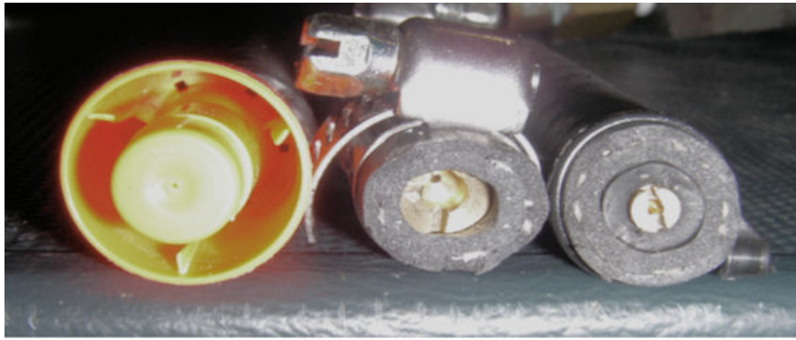
Figure 8 - Leak Orifices included a 1.0-mm Drilled Hole in a Plastic Cap, a 0.5-mm Carburetor Main Jet, and a 0.3-mm Carburetor Air Jet
