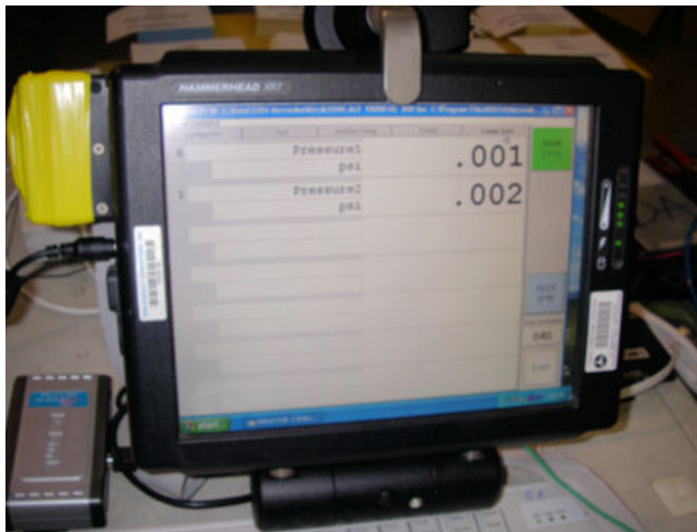
Figure 9 - A Tablet PC was used for Instrumentation Setup, Data Collection, and Real-Time Display of the Tank Pressure
