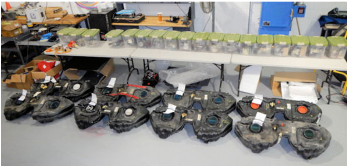
Figure 1 – The Fuel Tank Components were Labeled, Inspected, and Photographed before Testing
