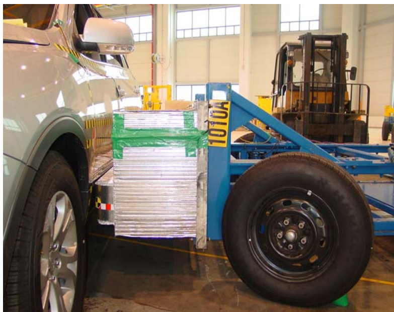
PRE-TEST : FRONT VIEW OF IMPACTOR FACE
