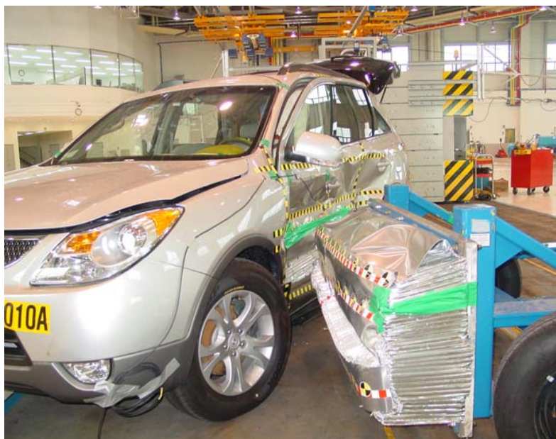
POST-TEST : FRONT VIEW OF IMPACTOR FACE
