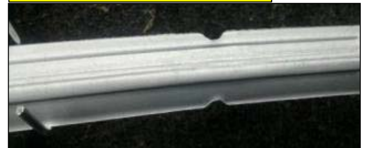
NG : Insufficient spray(overall)
