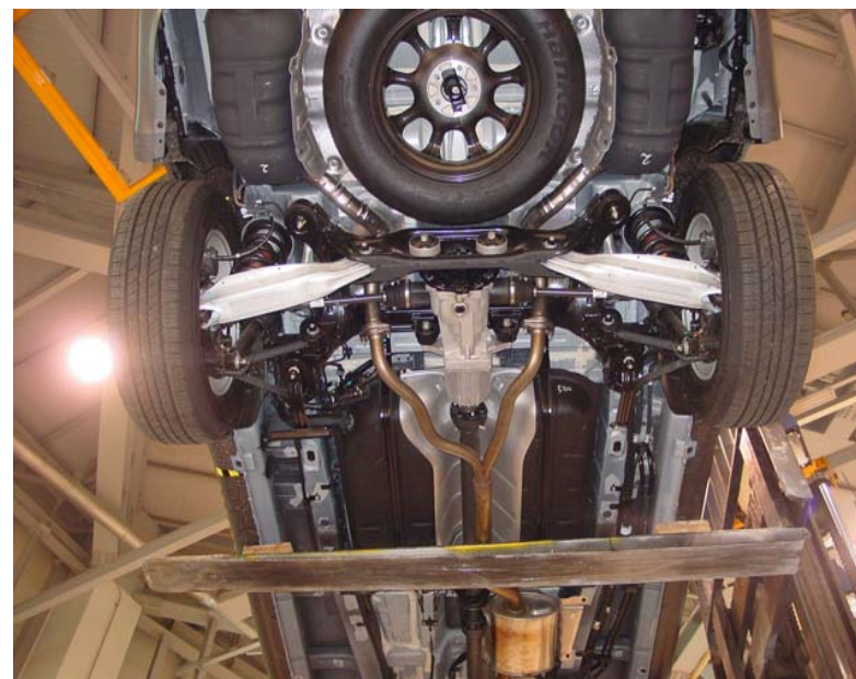
PRE-TEST : REAR UNDERBODY VIEW OF VEHICLE
