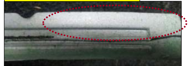
NG : Partial Insufficient spray
