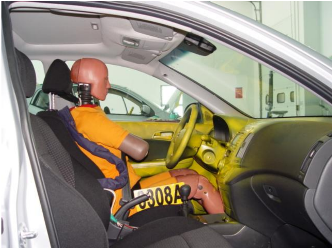
13. Pretest Driver Dummy View
