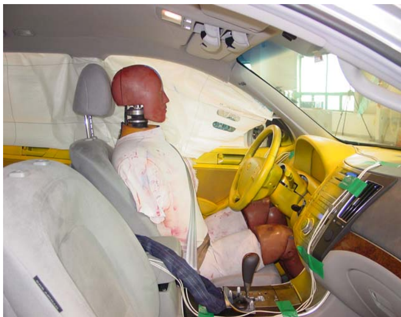
POST-TEST : OCCUPANT COMPARTMENT VIEW SHOWING FRONT SID
